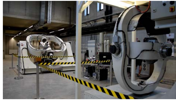
Fig. 4. High precision, high dynamics turntables for testing relative attitude motion in the satellite formation for intersatellite links and for joint observations.
