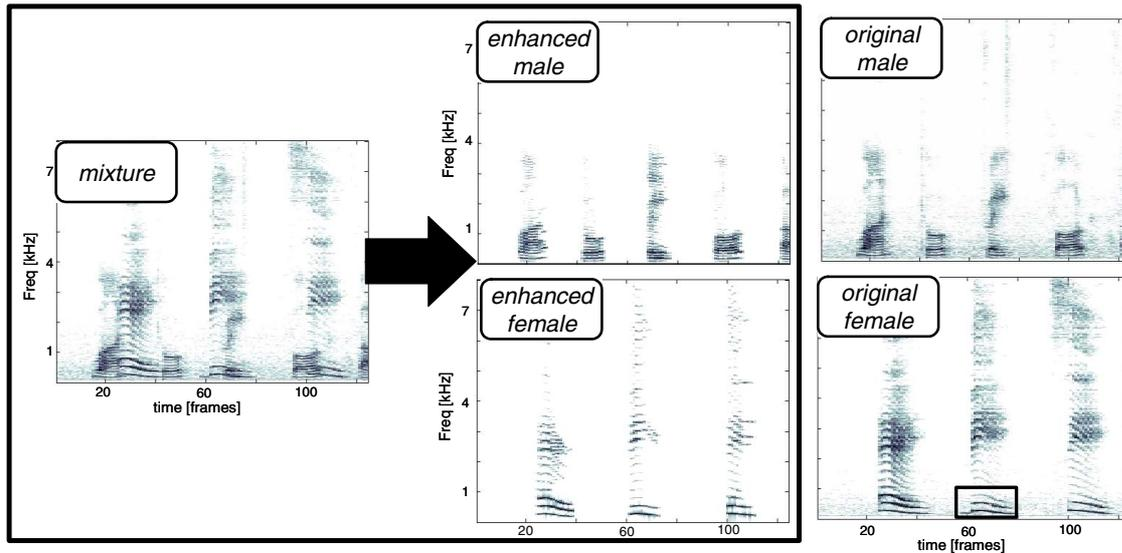
Figure 5. Spectrograms corresponding to the `speakers` sequence. Based on *visual* data, the audio components of each of the speakers were automatically separated from a single soundtrack. A small section in the original spectrogram of the female is marked. It was zoomed-in in Fig. 3.
