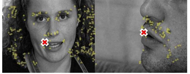
Figure 4. A frame from the speakers sequence. Out of the selected and tracked visual features [Dots], two are automatically associated to the audio [Crosses]: correctly, one per source. The audio mixture is also decoupled to two separate speakers.
