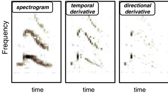
Figure 3. [Left] A section of a spectrogram (female speaker) exhibiting a frequency drift. [Middle] A temporal derivative (Eq. 12) results in high values through the entire sound duration. [Right] The directional derivative (Eq. 14) handles the frequency drift well. Resulting high values occur mainly at the onset.
