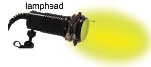
Fig. 2. Illustration [16] of an anisotropic illumination pattern  $Q(\mathbf{X})$ . Even in the same radial distance from the lamphead, the lighting changes laterally.
