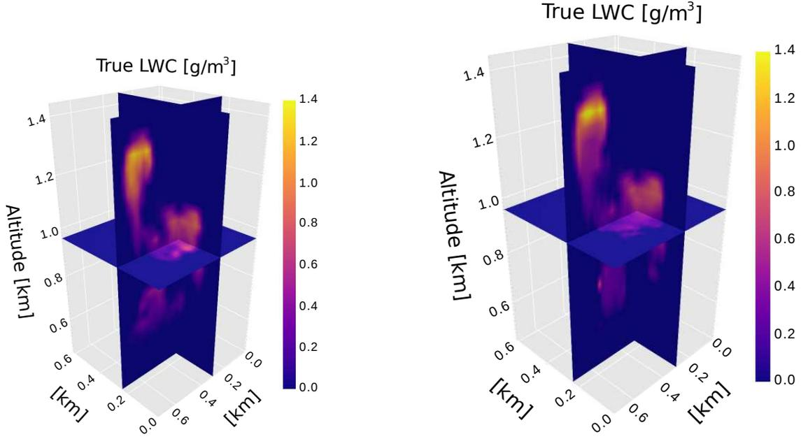
Figure 9: **Scene A** recovery results. [Left] Slices of the true cloud generated by LES. [Right] Slices of the cloud estimated tomographically using AirMSPI polarized bands.
