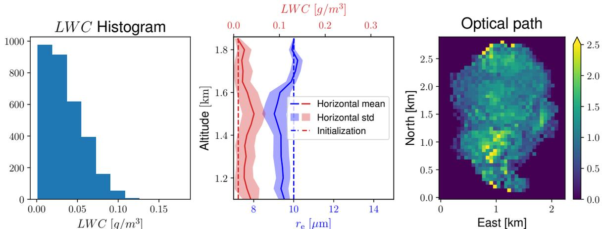
Figure 12: [Left] Following Yum et al.,<sup>44</sup> the recovered LWC is thresholded at  $0.001 \text{ g/m}^3$  in this histogram. [Middle] The profiles of mean and standard deviation of both LWC and  $r_e$  are plotted along with the respective choices of initial guess. [Right] Vertically-integrated optical thickness from the recovered extinction mapped at the pixel scale.
