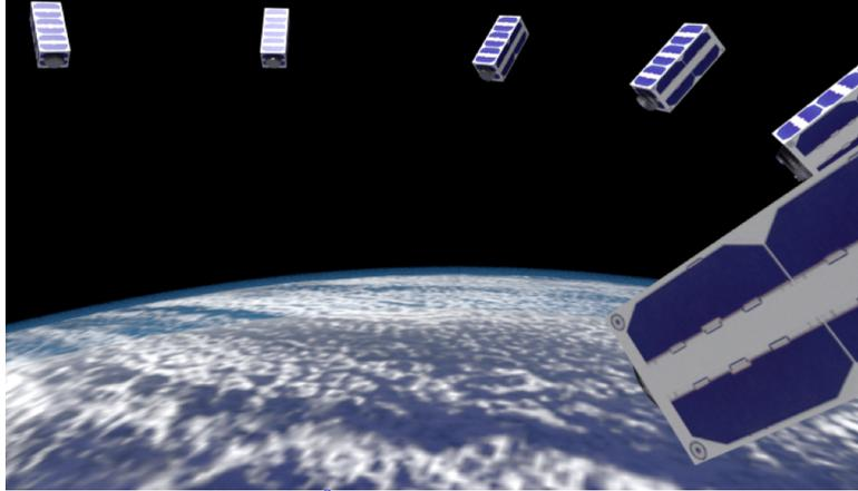
Figure 1: Artist’s illustration of the CloudCT<sup>8</sup> mission: a distributed multi-view system of 10 nano-satellites orbiting the Earth in formation. Measurements acquired by the formation will enable tomographic retrievals of cloud properties.
