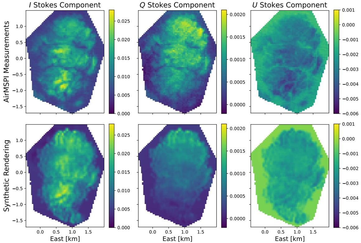
Figure 13: [Top row] 29.1°-aft AirMSPI measurements of Stokes vector components ( $I, Q, U$ ), from left to right, that are *not* used in the tomography. [Bottom row] Same as top row, but rendered by vSHDOM using LWC and  $r_e$  fields recovered using the 8 other views and the prescribed  $v_e = 0.1$ .
