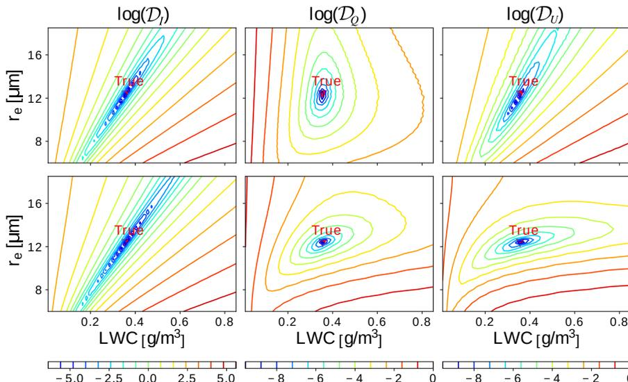
Figure 6: Logarithm of the 2D cost manifolds for the two-parameter homogeneous cubic cloud in Fig. 5. Each column of plots corresponds to the cost of the different Stokes components in Eqs. (20)–(22). Each row of plots corresponds to a different solar azimuth angle  $\phi_0$ .
