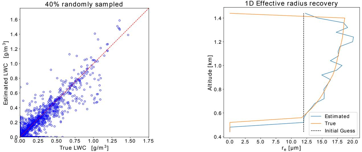
Figure 10: **Scene A** recovery results. [Left] Scatter plot of estimated vs. true LWC. The correlation coefficient is 0.94. [Right] recovery results of the 1D effective radius.
