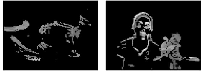
Fig. 7. Dynamic pixels expressed by the wavelet components in [left] Movie #1 and [right] Movie #2. Gray levels indicate the temporal average of pixel values. Black regions represent static pixels.
