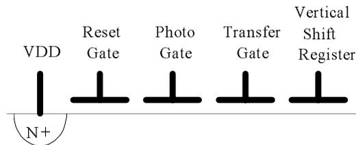
**Figure 3: CCD Sensor Cell Structure**
