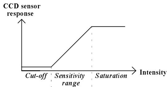
**Figure 1: The response of a CCD sensor**
