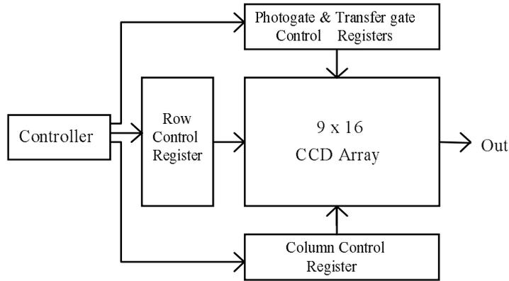
**Figure 2: The A/S CCD Imager Chip Architecture**
