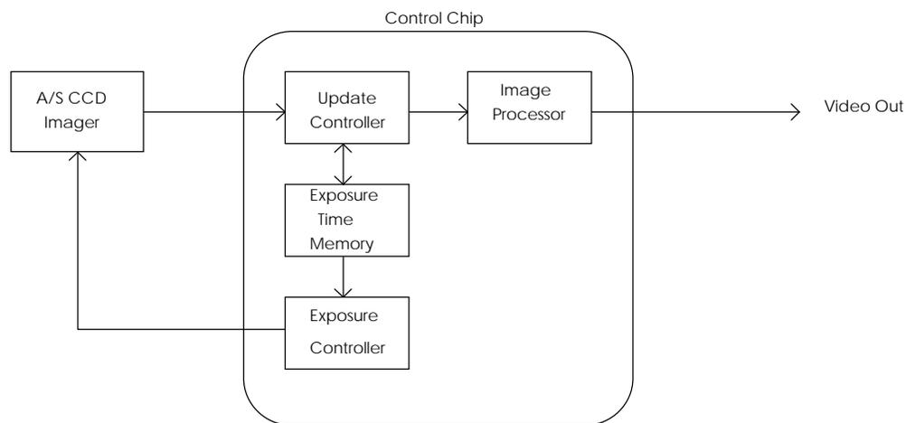
**Figure 5: System Architecture**
