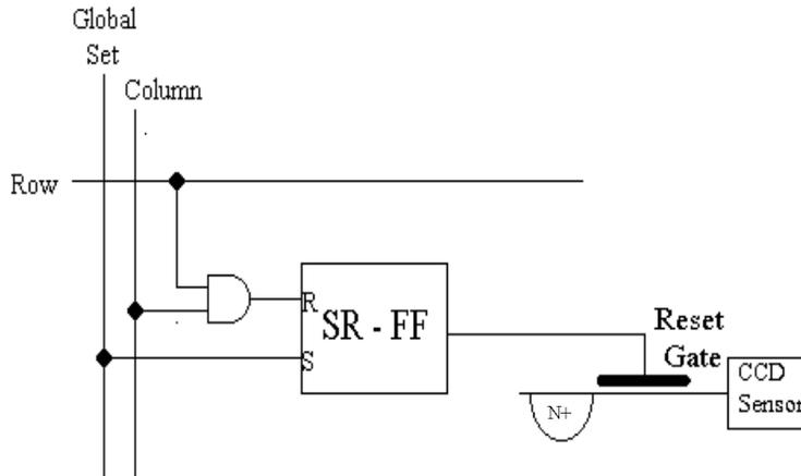
**Figure 4: Reset Gate Control**
