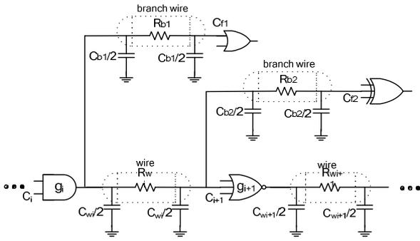
Fig. 9. A logic path segment including RC interconnect and two branches.  $R_b$  and  $C_b$  are the resistance and capacitance of branch wires, respectively, and  $C_f$  is the fanout load capacitance.
