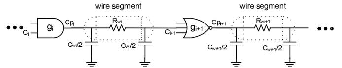
Fig. 2. Cascaded logic gates with resistive-capacitive interconnect.
