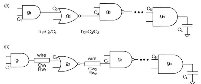
Fig. 1. Cascaded strings of logic gates. (a) Logical effort optimization for gates without wires is based on equal stage efforts, e.g.,  $g_1 h_1 = g_2 h_2$ . (b) In the case of gates with wires, the rule of equal effort breaks down due to fixed wire parameters.
