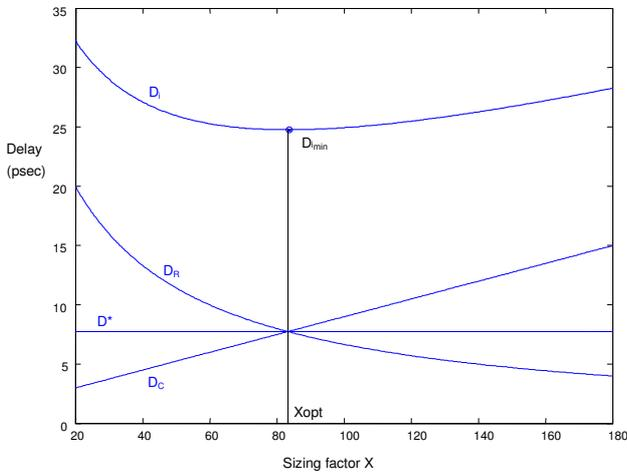
Fig. 4. Dependence of delay on the sizing factor (for a NAND gate with  $L_i=100 \mu m$ ,  $L_{i-1}=1 mm$ ,  $C_{i-1}=C_0$ , and  $C_{i+1}=10C_0$ ).
