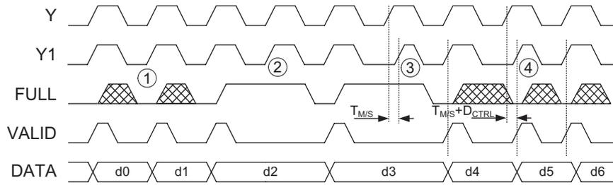
Fig. 13. LDL output port operation.
