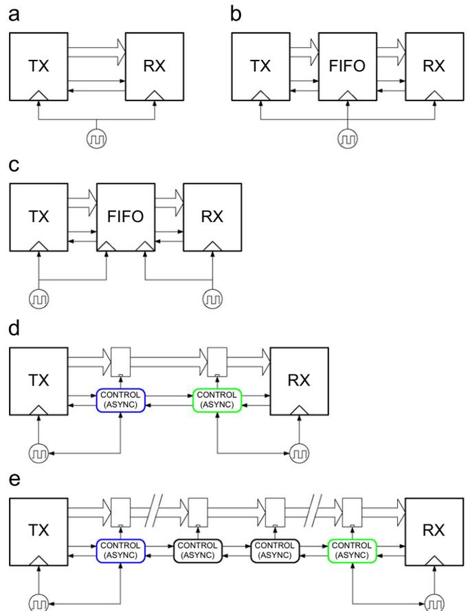
**Fig. 3.** Fast synchronization: (a) single clock domain transfer, (b) buffered single clock domain transfer, (c) two-clock FIFO synchronizer, (d) stoppable clock and LDL synchronizers and (e) synchronization over long interconnect.
