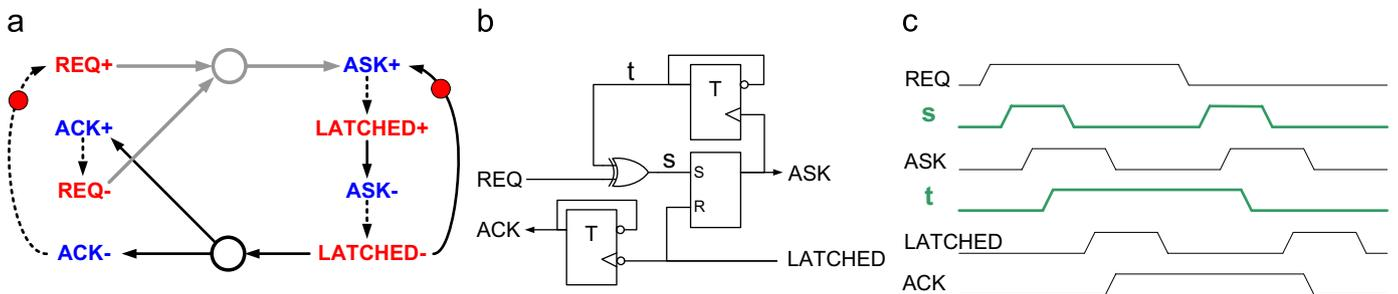
Fig. 8. Two-phase input-port asynchronous controller.
