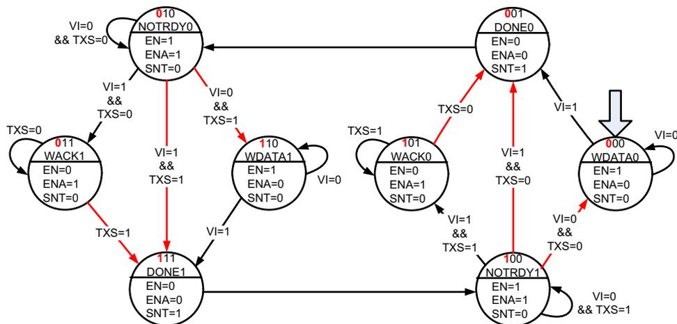
Fig. 2. TX FSM of the fast two-phase synchronizer.
