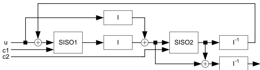
Figure 5: Iterative Decoder Detailed Scheme,  $I$  denotes interleaver
