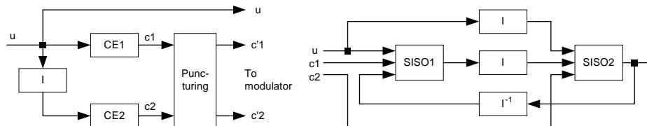
Figure 1 Turbo encoder and decoder,  $I$  denotes interleaver
