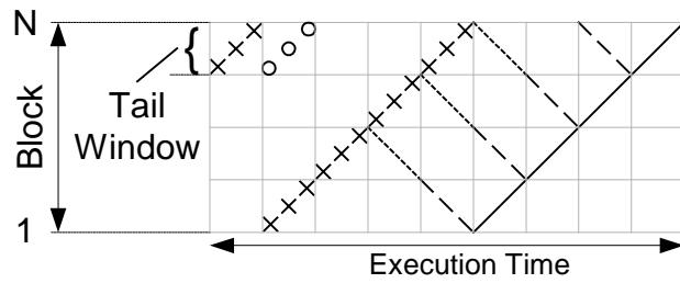
Figure 4: Sliding Window with Tailbiting SISO Algorithm
