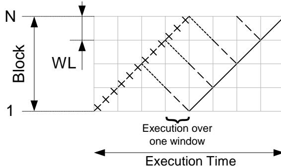
Figure 3: Sliding Window SISO Algorithm
