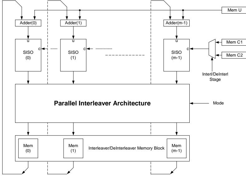
Figure 6: Parallel Decoder Architecture
