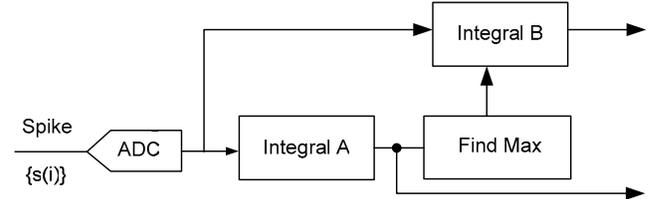
Figure 4: Digital MITA - VLSI architecture
