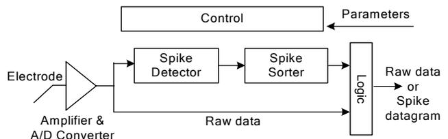
Figure 1: Neuroprocessor Architecture: one electrode section
