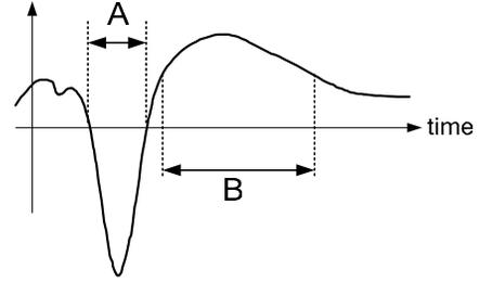
Figure 3: Two integration time intervals  $A, B$  for the IT D&A algorithm
