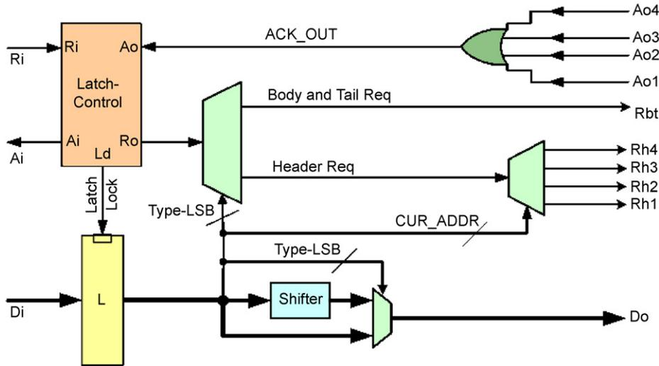
Fig. 9. Virtual channel input port (VC-IP) architecture.
