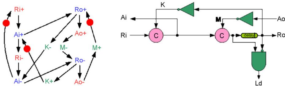
Fig. 10. Latch-control circuit and STG.
