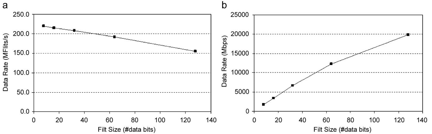
Fig. 19. Router throughput dependence on flit size: (a) flit rate, (b) bit rate.
