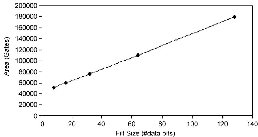
Fig. 20. Router cell area dependence on flit size.
