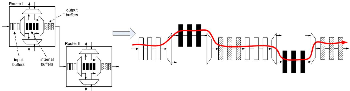
**Fig. 3.** NoC data path as pipeline.
