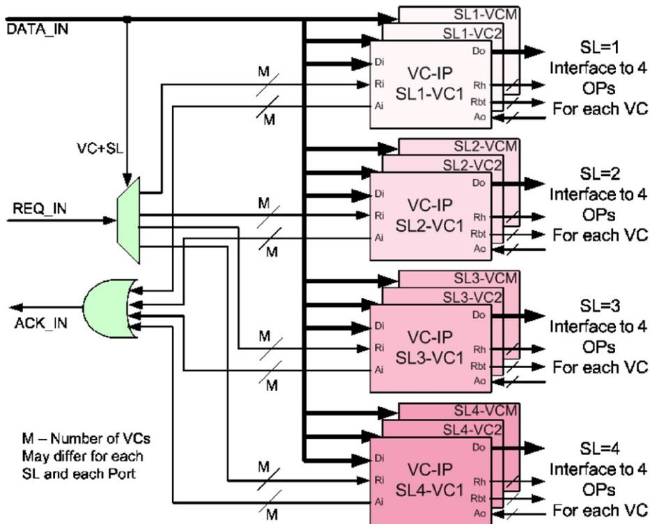
Fig. 8. QNoC multi-service levels router input port.
