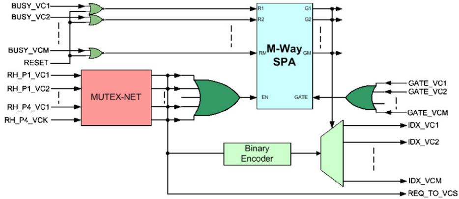
Fig. 13. Virtual channel admission control (VCAC) module.
