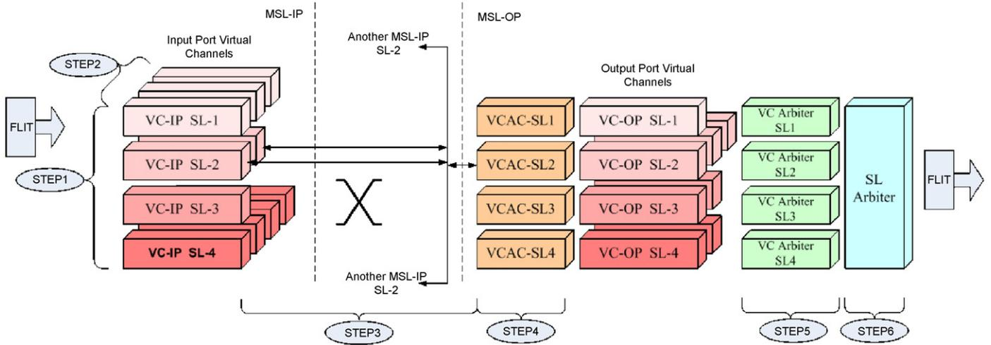
Fig. 7. QNoC router data flow.
