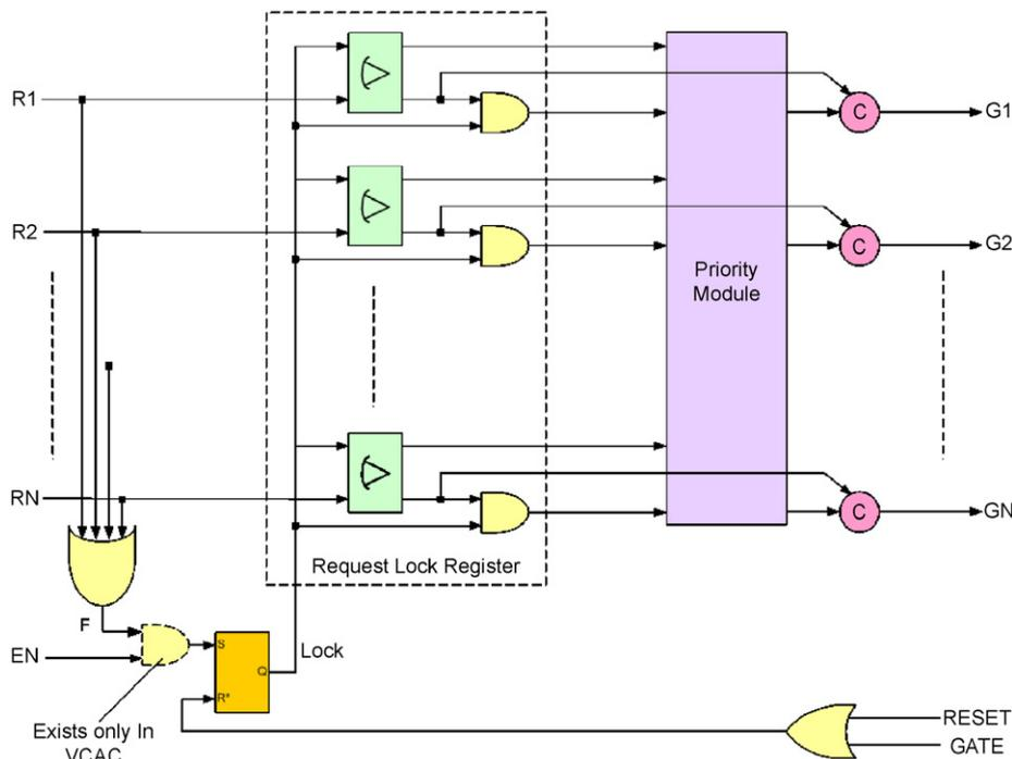
Fig. 12. *N*-way static priority arbiter.
