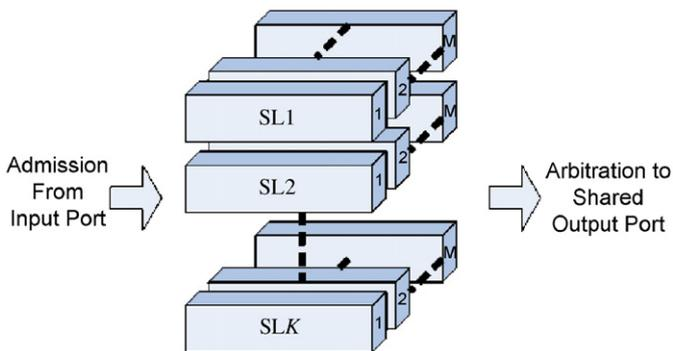
Fig. 2. Service level and virtual channels  $K$ —service levels,  $M$ —virtual channels ( $M$  can be different for each SL and port).
