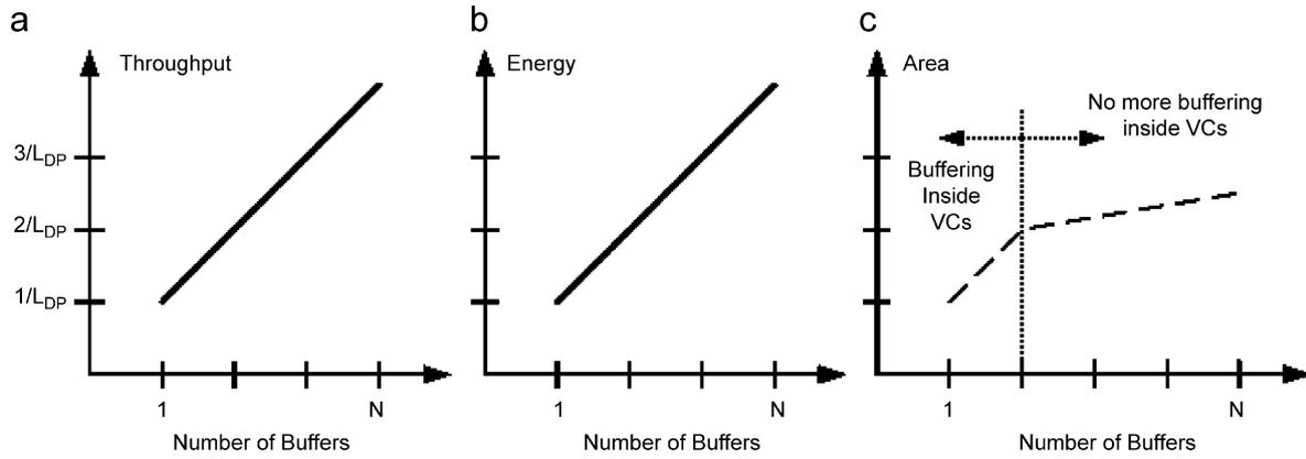
Fig. 4. Number of buffers impact on router performance.
