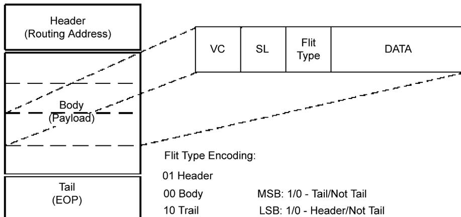
Fig. 6. Packet structure and flit format.
