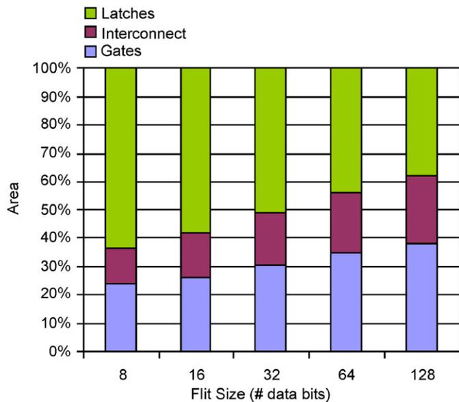
Fig. 21. Area distribution. Switching gates and wires dominate the area as flit size grows.
