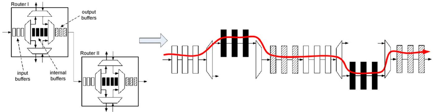
**Fig. 3.** NoC data path as pipeline.
