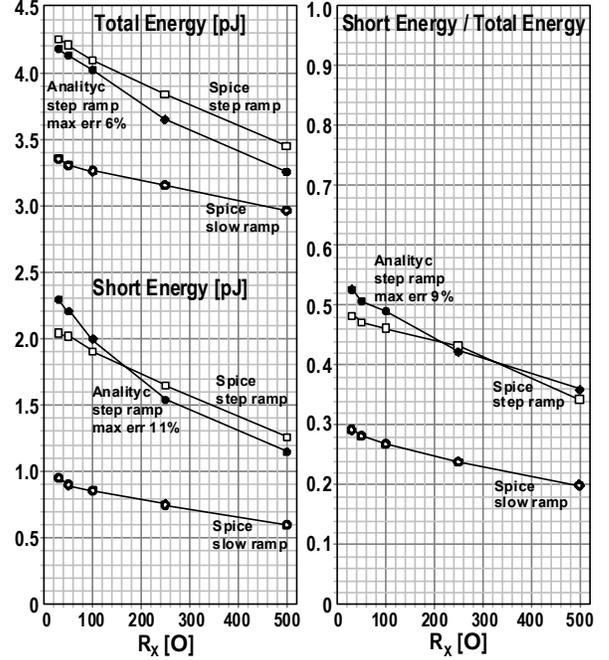
Figure 9: Total and short-circuit energy vs. crosslink resistance
