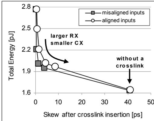
**Figure 10: Effect of crosslink on energy vs. skew for different values of  $R_X$  and  $C_X$ . The 40 ps skew without a crosslink, caused by either an unbalanced tree or due to misaligned inputs, is reduced by the crosslink.**
