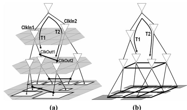
**Figure 1: Non-tree clock network topologies.**
