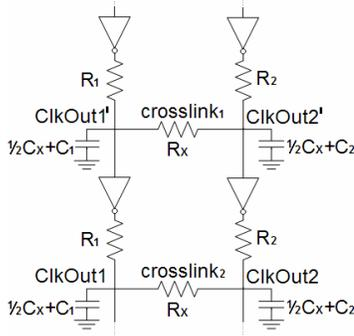
**Figure 11: Crosslink insertion at different tree levels**
