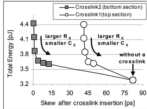
**Figure 12: Energy vs. skew for crosslink insertion at different tree levels. Inserting a crosslink at a higher level will usually achieve less skew reduction at the same energy due to the additional imbalance of loads, resistors, and drivers at the lower levels, affecting the delay.**
