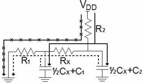
Figure 8: Current components for  $t \leq T$
