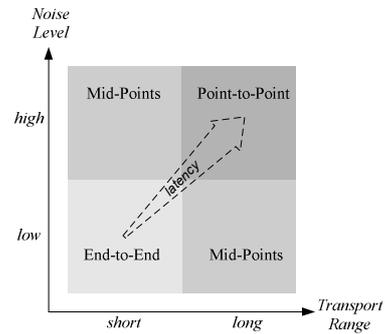
Figure 6. Micro-Modem application types.
