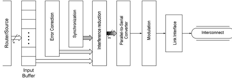
Figure 3. Transmitter architecture in the micro-modem concept
