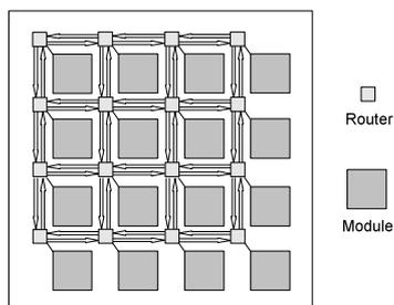
Figure 1. Typical Network on Chip structure.
