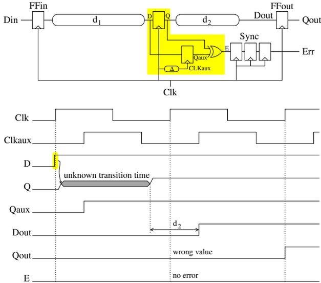
Fig. 1. Basic Razor scheme and timing diagram with a false positive.
