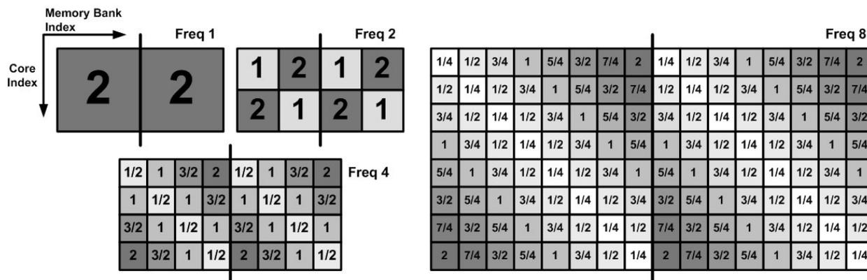
**Figure 4: ATM (Access Time Matrix) for different frequencies (normalized to freq1 cycles)**
