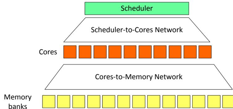
Figure 1: System architecture
