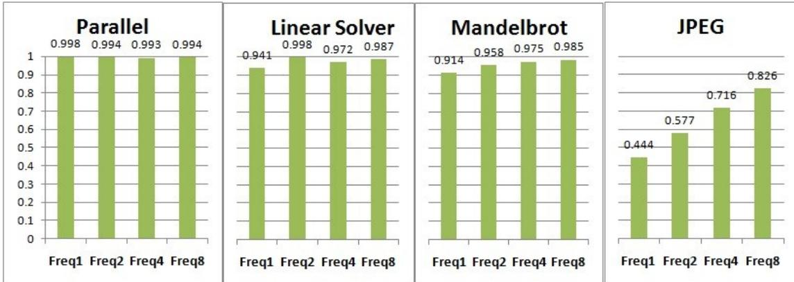
Figure 17: Network efficiency (non-equi-distant)
