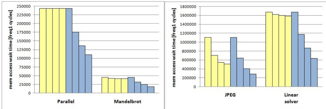
Figure 14: Memory access wait time comparison with 512 memory banks (each set of 4 bars corresponds to 4 frequency levels)
