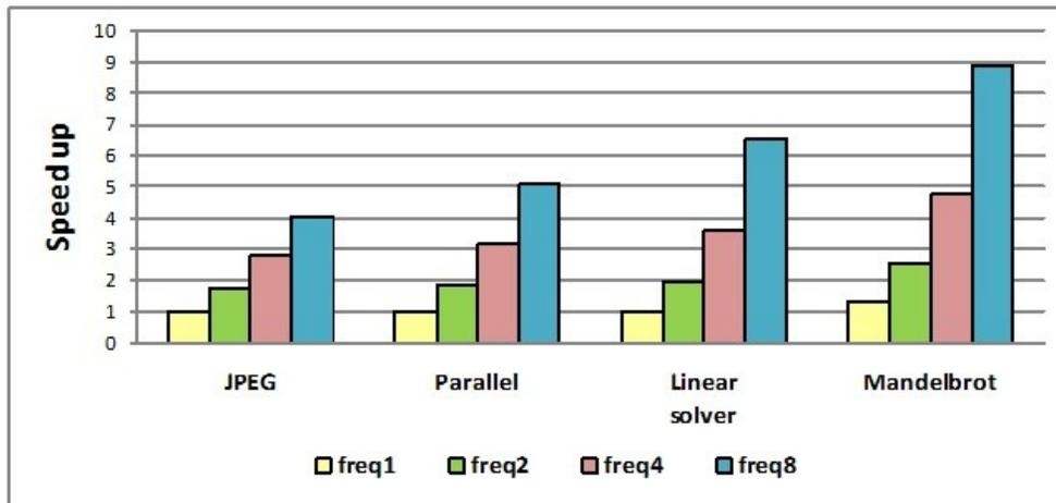
Figure 15: Benchmarks Speed-Up (non-equi-distance) with 512 memory banks
