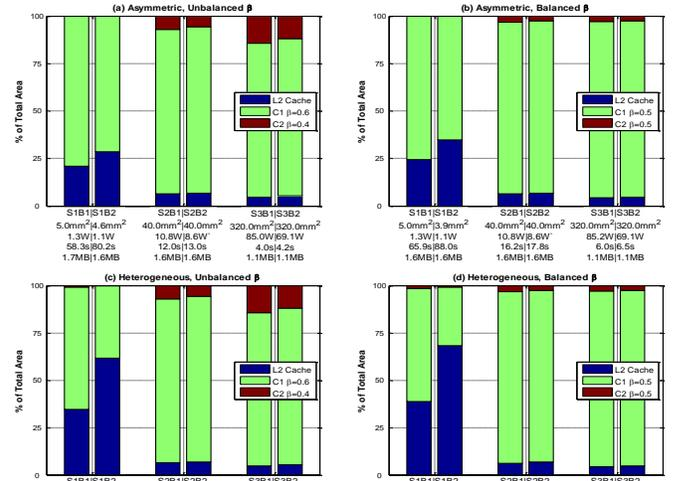
Figure 4. SoC area partitioning following optimization of execution time, subject to three scenarios of constrained resources.
