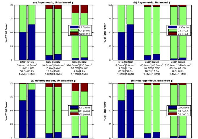
Figure 5. SoC power partitioning following optimization of execution time, subject to three scenarios of constrained resources.
