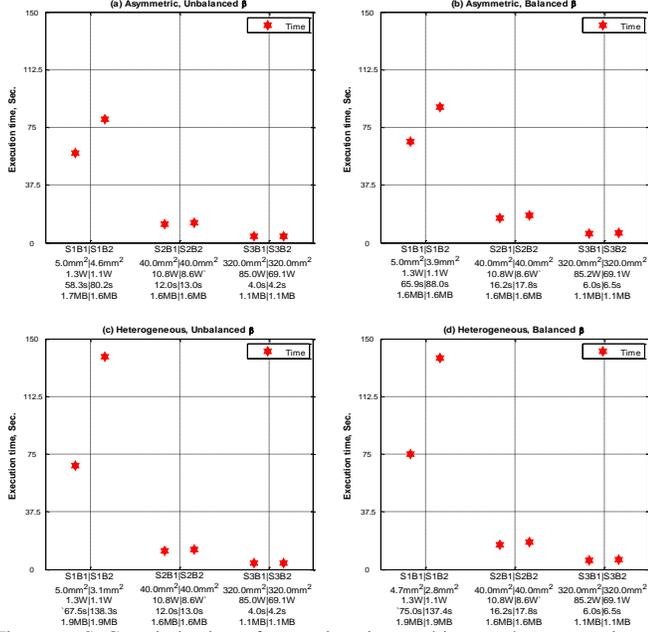
Figure 6. SoC optimization of execution time, subject to three scenarios of constrained resources.
