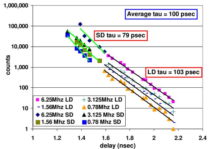
Figure 5 Metastability event counts as a function of resolution delay and the resulting synchronization time constant ( $\tau$ ) overall and region estimates for the regular library flip-flop circuit.
