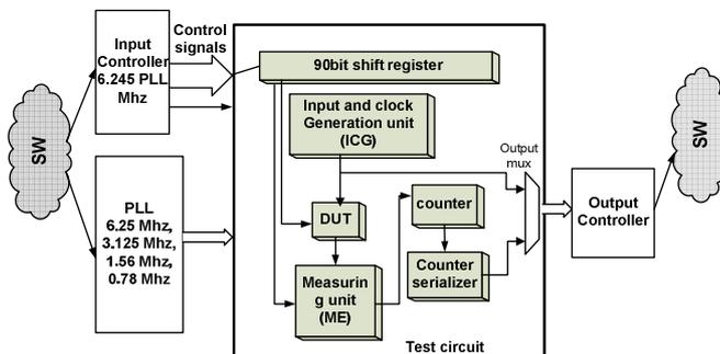
Figure 3. Block diagram of the metastability measurement circuit and system.
