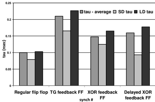
Figure 7 Metastability resolution performance comparison of the tested flip-flop circuits.
