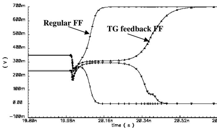
Figure 8 Simulation result of the regular FF and feedback FF
