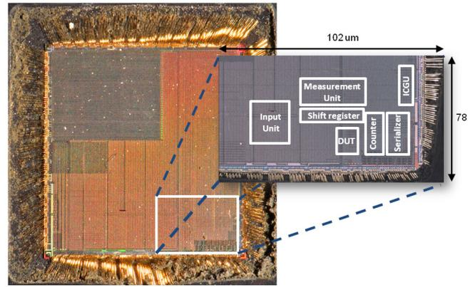
Figure 9. Micrograph of the metastability measurement circuit fabricated in 65nm CMOS.
