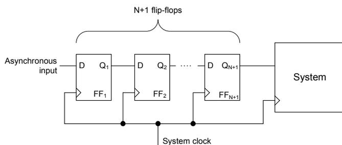
Figure 1. A typical synchronizer using N+1 cascaded flip flops
