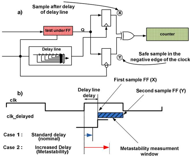
Figure 2 (a) Metastability measurement method (b) Waveforms explaining the operation of measuring method.
