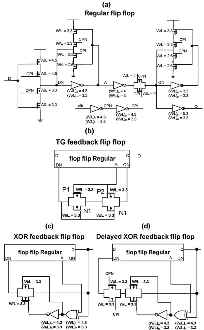
Figure 4. Schematics of the tested synchronization flip-flop circuits (a) regular library FF (b) TG feedback FF (c) XOR feedback FF (d) Delayed XOR feedback FF.
