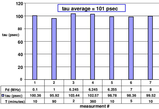
Figure 6. Measured  $\tau$  for different data frequencies, and measurement periods of the regular library flip flop.
