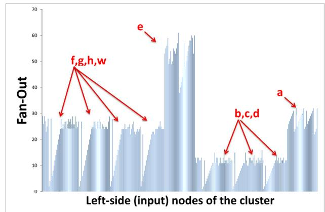
Fig. 8. Histogram of fan-outs for the left-side nodes connecting to the sample cluster of the right-side nodes. Eight groups, corresponding to the eight 32-bit stage input words, can be clearly seen. The fan-out can be used to associate the groups with specific words.
