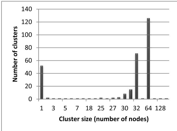
Fig. 6. Histogram of cluster sizes in the Bitcoin SHA-256 accelerator. The biggest group includes clusters with 64 nodes; hence, it matches the compression stages. The second biggest group includes clusters with 32 nodes; hence, it matches the message schedule stages.
