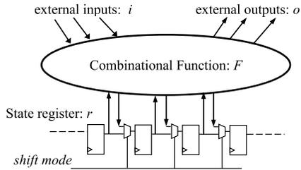
Fig. 1. Scan Design. Scan insertion adds multiplexers to each flip-flop in the chip, so that when shift mode is on, all the flip-flops are accessible from off-chip via a serial channel. The combinational function  $F$  represents the collection of combinational logic cones connecting flip-flops to one another and with primary inputs/outputs.
