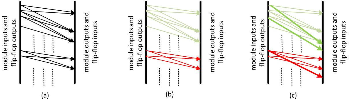
Fig. 3. Directed bipartite partial dependence graph. (a) After the run of the junta algorithm. (b) After SNN clustering (colors designate clusters). (c) After completing missing dependencies (bold lines indicate newly added edges).
