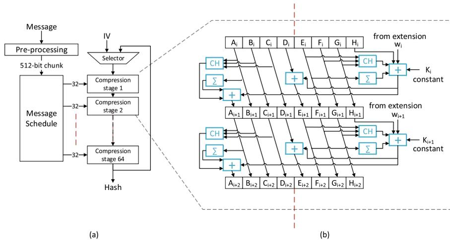
Fig. 2. SHA-256 algorithm block diagram. (a) SHA-256 execution flow, including preprocessing stage, message schedule, which outputs  $64 \times 32$  bit words, and 64 compression stages. (b) Detailed diagram of two 256-bit-wide compression stages. Each includes  $6 \times 32$  pass-through connections, two 32-bit adders, one five-element, and one seven-element. In addition, the compression stage includes permutations, selectors, and majority functions.
