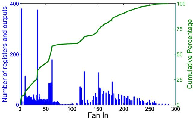
Fig. 4. Transitive fan-in histogram for flip-flop inputs and primary outputs in the ITC'99 benchmark circuits. About 50% of them have fan-in of 50 or less. Peaks can be seen at fan-ins that are multiples of 32, hinting about processor registers and arithmetic circuits.
