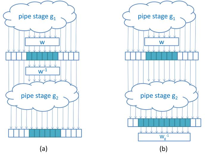
Fig. 5. Embedding the PAW watermark in pipeline stages. (a) First-order watermark comprises the encoder  $w$ , which encodes the pipe stage register inputs and the decoder  $w^{-1}$ , which is attached to the pipe register output and implements the inverse transformation. (b) Second-order watermark in which the decoder is attached to the next pipeline stage. The decoder performs a more complex transformation that includes the function of the pipeline stage.
