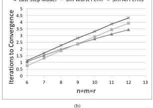
Fig. 9. (a) The dependency on r of the number of iterations to convergence for p = 1 and constant m = n = 6. (b) Comparison of time to convergence for Clos(n = m = r) in the case of half-link-rate flows (p = 2) using the Last-Step Model and a dedicated simulation model.
