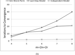
Fig. 8. Expected convergence time for p = 1, i.e. at most one flow per link. The plots compare the approximations of the Independent single-outputswitch model and the Last-Step model, against simulated results of worst permutations, in the cases where (a) the topology is rearrangeable nonblocking with m = n = r. and (b) the topology is strictly non-blocking with m = 2n = 2r.
