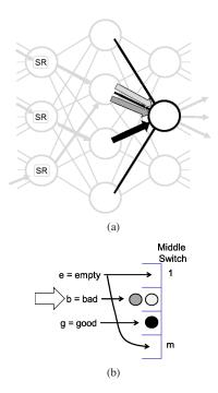
Fig. 2. A balls-and-bins representation: (a) A single output switch of the Clos network with 2 flows contending on its second link from the top. (b) A balls-and-bins representation of the m output-switch input links as bins and the n flows as balls. For the case where the bandwidth of each flow equals the link bandwidth (p = 1), the state variable e represents the total number of empty bins, b the number of bad bins and g the number of good bins.
