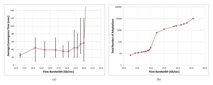
Fig. 11. Simulated cluster of 1152 nodes, running a a set of random permutations of 256KB for different flow bandwidths. (a) shows the average and range of convergence time from the start of the permutation period. It can be seen that flow bandwidth above half the link bandwidth simply does not converge. (b) depicts the total number of adaptations throughout the entire simulation period on a logarithmic scale.
