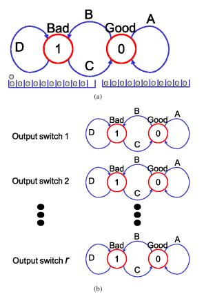
Fig. 5. Approximated Last Step model of a single output-switch: (a) A single bad state implies a lower bound on convergence time as it does not let the bad state degrade further than the last step. (b) The set of r state pairs describes the entire system.
