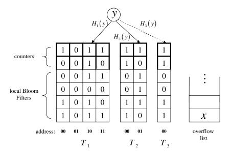
Figure 1: Illustration of a Balanced Bloom Filter implementation based on MHT, with three subtables.
