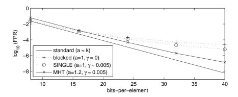
Figure 5: False positive rates of different Bloom Filter schemes with memory block size of B=256 bits and variable load r. SINGLE and MHT use overflow fraction  $\gamma\approx0.5\%$ .
