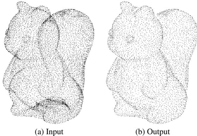
Figure 1. **Given points sampled from a surface and a viewpoint** (a), only the points that would be visible if the surface were known, are extracted (b).
