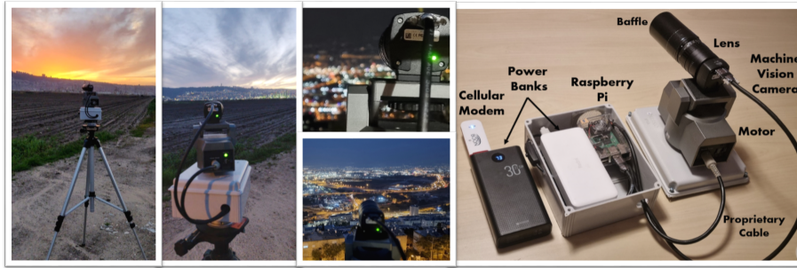
Fig. 9. [Left] Sample images from the outdoor experiment. [Right] A custom-built imager. It consists of an industrial camera, a C-mount lens, a raspberry-pi controller and a motorized pan and tilt head.
