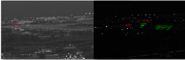
Fig. 1. Scintillating light sources over Haifa Bay, imaged on a winter evening. [Left] A preliminary capture of a twilight scene consists of lights and landmarks. [Right] Operational imaging optimized for turbulence scintillation sensing. Colors encode processed results: valid measurements are in green; red denotes signals that are either saturated or too dim.
