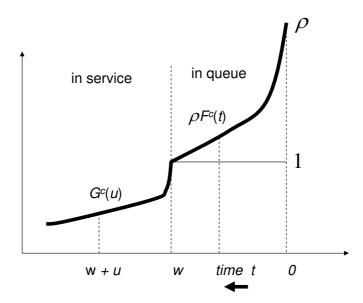
Figure 1: The steady-state density of fluid content as a function of total time t in system, with t increasing to the left, for the G/GI/s+GI fluid model with service rate 1, arrival rate  $\rho>1$ , service-time cdf G, time-to-abandon cdf F and no delay announcement.
