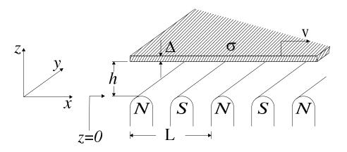
Figure 7.14: Metallic plate moving above an array of periodic magnets.
