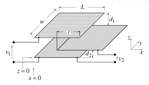
Figure 5.2: Simple electro-static coupling example.
