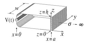
Figure 4.2: Model of a quasi-static inductor.
