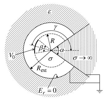
Figure 7.12: Resistor with an "edgy" electrode.
