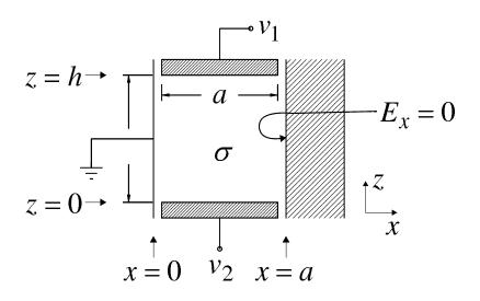
Figure 5.13: Simple model for conductive coupling.
