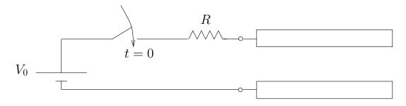
Figure 4.7: Charging of a lumped capacitor.
