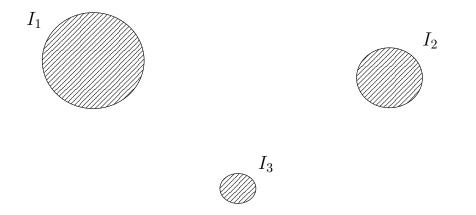
Figure 5.15: Three wires with the third providing the return path to the other two currents.
