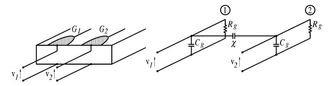
Figure 5.7: Two gates that may become coupled (left) and the equivalent circuit that describes their operation.
