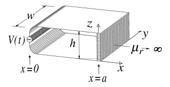
Figure 4.1: Model of a quasi-static capacitor.
