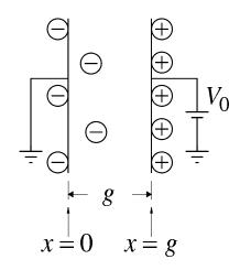
Figure 7.B.1: Vacuum diode.
