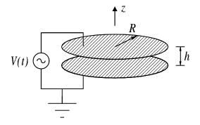
Figure 3.1: Simple model for a capacitor.
