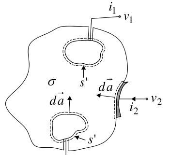
Figure 5.12: Schematics of a system characterized by stationary conductive coupling.  $\overline{-}$
