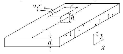
Figure 7.4: The magnetic flux imprinted in a moving tape is measured as voltage by a suspended loop.
