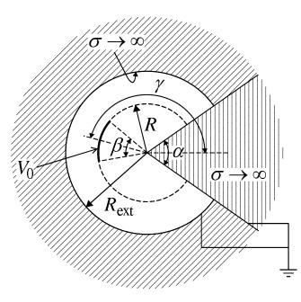
Figure 7.9: Capacitance associated with an edge.
