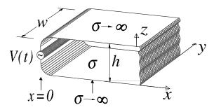
Figure 4.3: Model of a quasi-static resistor.
