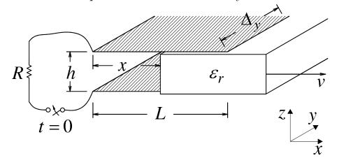
Figure 7.3: A dielectric layer moves between the two plates of a capacitor.
