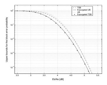
Fig. 3. Various upper bounds on the block error probability of the ensemble of serially concatenated codes depicted in Fig. 2. The compared bounds are the tangential-sphere bound (TSB) and the union bound with and without expurgation of the distance spectrum; this expurgation refers to the ensemble of inner codes, chosen uniformly at random from the ensemble of (8,7) binary linear block codes.
