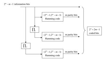
Fig. 6. A multiple turbo-Hamming encoder. The encoder consists of parallel concatenated Hamming codes with two uniform, statistically independent interleavers. The code length is  $2^m + 2m - 1$  and the code rate is  $R = \frac{2^m - m - 1}{2^m + 2m - 1}$  bits per channel use.
