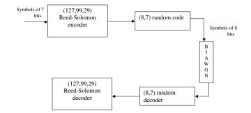
Fig. 2. A scheme for an ensemble of serially concatenated codes where the outer code is a (127, 99, 29) Reed-Solomon (RS) code, and the inner code is chosen uniformly at random from the ensemble of (8,7) binary linear block codes.
