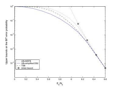
Fig. 5. Comparison between various upper bounds on the ML decoding bit error probability of the ensemble of (1033,1013) uniformly interleaved turbo-Hamming code. The compared bounds are the union bound (UB), the tangential-sphere bound (TSB), the upper bound from Theorem 3.3 which combines the union bound with the MSFB (UB+MSFB), and the upper bound from Theorem 3.4 which combines the union bound with the simplified DS2 bound (UB+simplified DS2).
