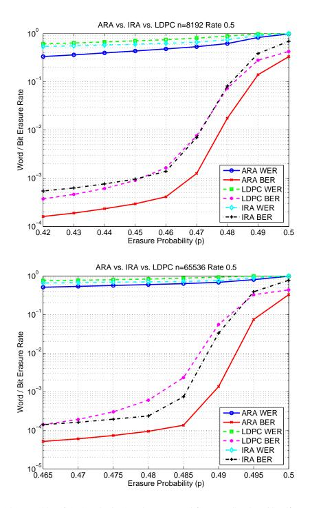
Fig. 8. Simulations for the ensembles of ARA and NSIRA codes constructed from LDPC codes with self-matched degree distributions (see Sections VI-A and VI-B), and the ensemble of right-regular LDPC codes in [3]. The plots refer to block lengths of 8192 and 65536 bits (see upper and lower plots, respectively) and a design rate of 0.5 bits per channel use. No high-rate outer code is assumed.
