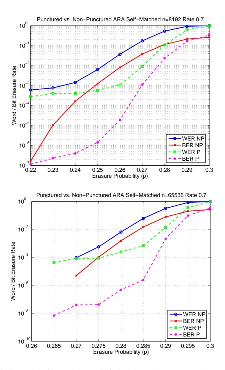
Fig. 12. Simulations for the ensemble of punctured ARA codes in Section VI-A where we compare the case where the self-matched ensemble is designed directly to a rate of 0.7 bits per channel use, versus the case of designing the ensemble for a rate of 0.5 and increasing the rate by puncturing. The upper and lower plots refer to block lengths of 8192 and 65536 bits, respectively. P and NP stand for 'punctured' and 'non-punctured'.
