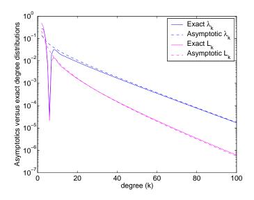
Fig. 7. A plot comparing the asymptotic versus exact expressions of the degree distributions  $\{L_k\}$ ,  $\{R_k\}$ ,  $\{\lambda_k\}$  and  $\{\rho_k\}$  of the selfmatched ARA ensemble, designed for a BEC with erasure probability of  $p = \frac{1}{2}$ . The parameter b in the left and right degree distributions (45) and (46), respectively, is determined by Eq. (48), so its value is b = 0.9304.
