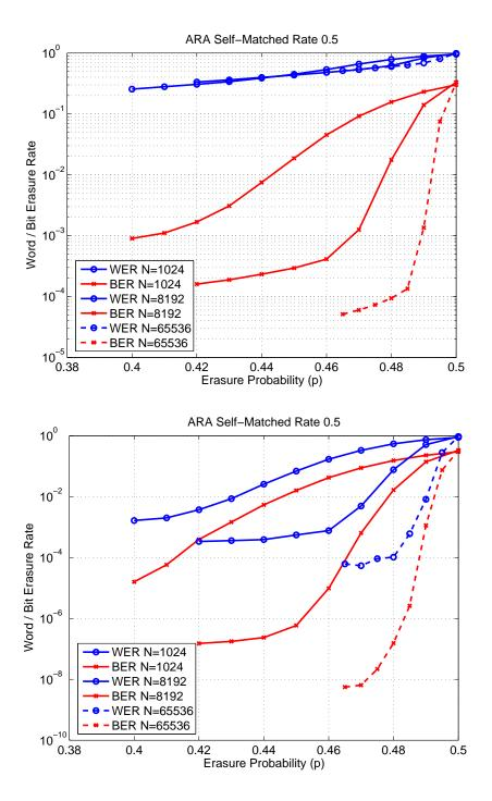
Fig. 10. Simulations for the ensemble of ARA codes in Section VI-A, constructed from the ensemble of LDPC codes whose degree distributions are matched to themselves. The design rate of the ensemble is 0.5 bits per channel use. The upper plot refers to the case where there is no outer high-rate code, and the lower plot refers to the case where there is such a code.
