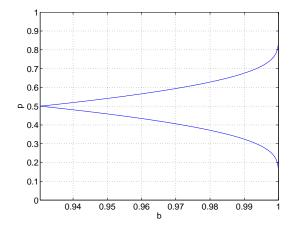
Fig. 4. Valid values of p as a function of the parameter b in (45) and (46), so that the coefficients in the power series expansions around zero of  $L(\cdot)$ ,  $R(\cdot)$ ,  $\lambda(\cdot)$  and  $\rho(\cdot)$  are all non-negative. This region is determined by the inequalities in (47), and it is therefore bounded by the upper and lower curves in this figure.
