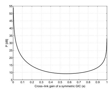
Fig. 1. The curve in this figure shows the threshold for the SNR (P), in decibels, as a function of the cross-link gain (a) for a weak and symmetric GIC. This threshold is given by the right-hand side of (19). For points (a, P) above this curve, the ETW bound is better in providing an upper bound on the corner points of the capacity region, whereas Kramer's bound is better in this respect for points (a, P) below this curve.
