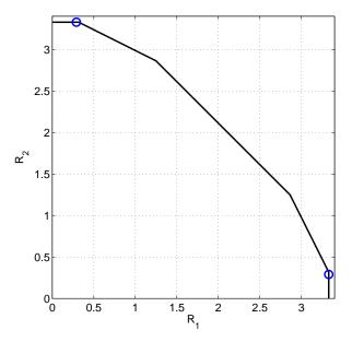
Fig. 2. The figure refers to a GIC with cross-link gains  $a_{12} = a_{21} = 0.5$ , and a common transmitted power  $P_1 = P_2 = 100$  in standard form (see Example 2). The solid curve is the boundary of the outer bound in [10, Theorem 3] (the ETW bound in (20)), and the two circled points refer to Conjecture 1; these points are achievable, and they almost coincide with the boundary of the outer bound.
