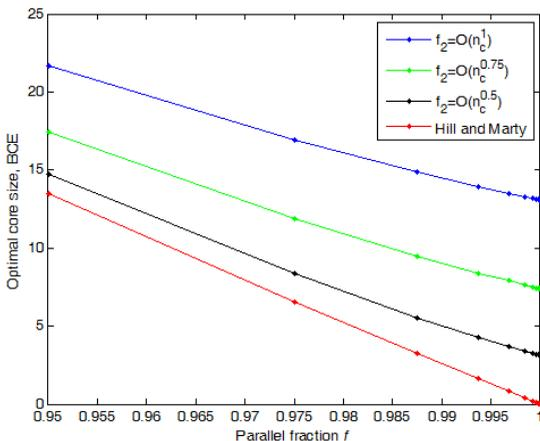
Figure 13. Optimal symmetric core size vs.  $f$  for various values of  $f_2$
