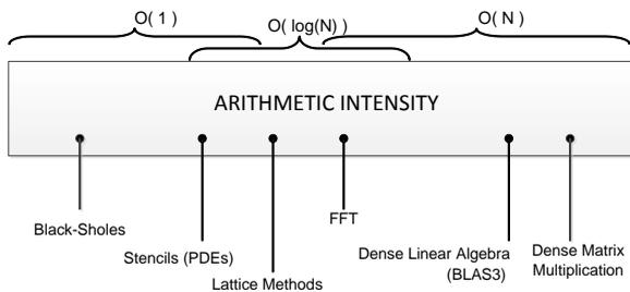
Figure 4: Arithmetic Intensity [26].
