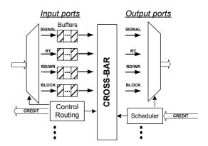
Figure 2. QNoC Router Architecture
