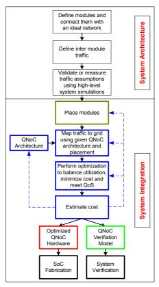
Figure 3. System development flow with QNoC
