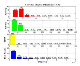
Figure 6. QNoC Simulation results: distribution off endto-end (ETE) delay for each SL -used for links capacity allocation and statistically ensures that 99.9% of the packets are provided the required QoS.
