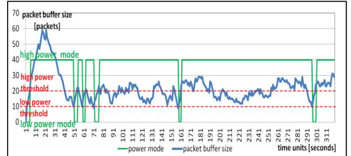
Figure 2. Packet buffer simulation
