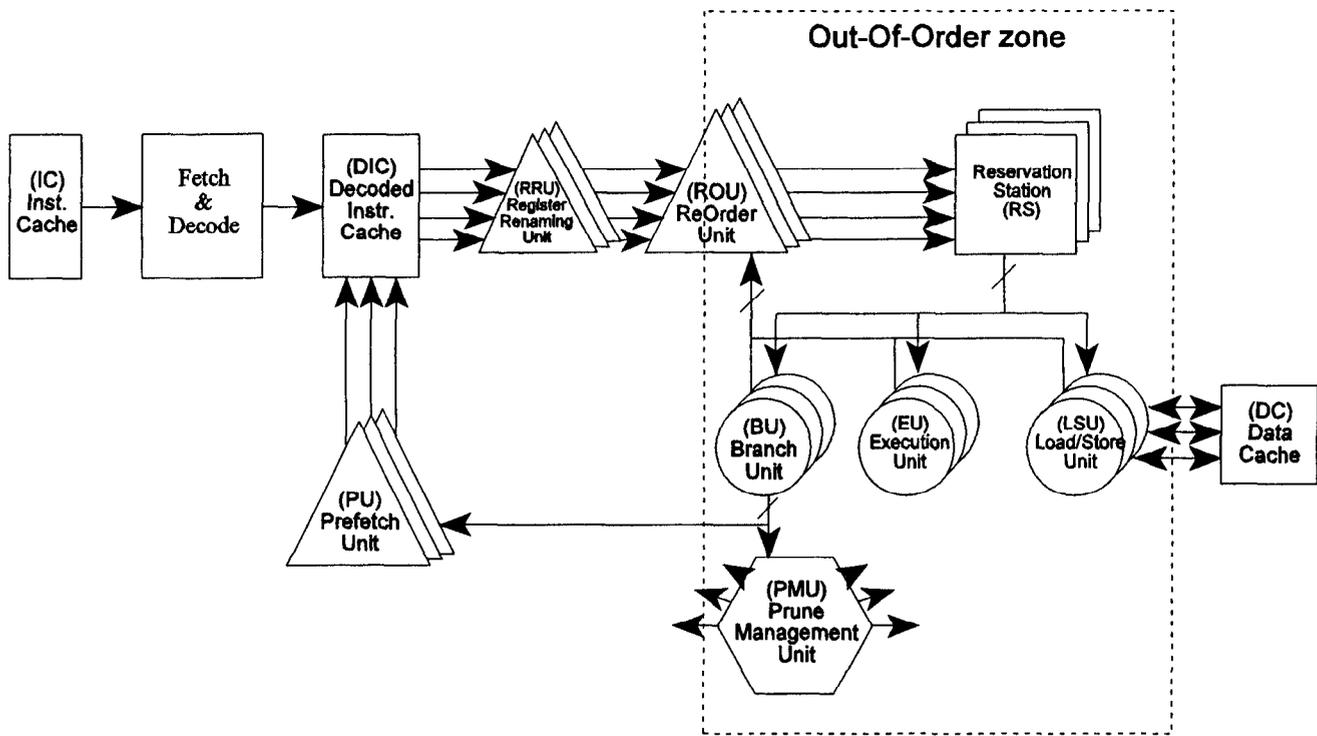
Figure 1: *Kin* asynchronous processor architecture.
