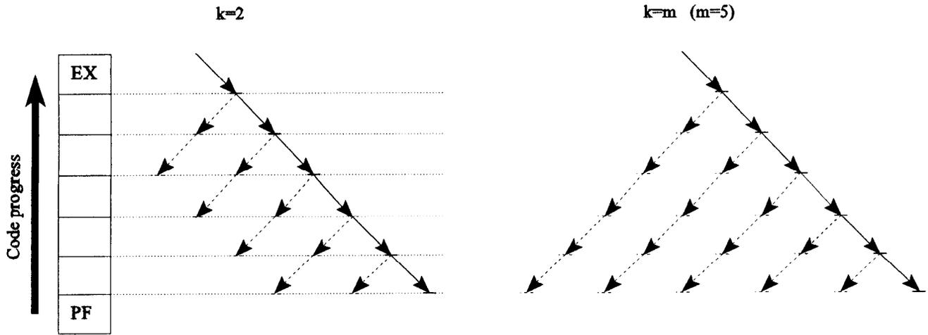
**Figure 3:** Examples of *Avid* Execution depth ( $k$ ).  $m$  is the number of processor pipeline stages between prefetch (PF) and branch resolution (EX) stages.
