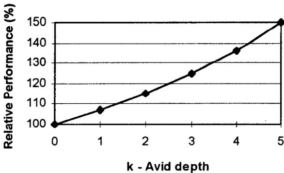
**Figure 4:** Average performance improvement achieved by various Avid depths ( $k$ ), for  $m=5$ ,  $p=0.95$ , and high bandwidth (execution limited by ILP).
