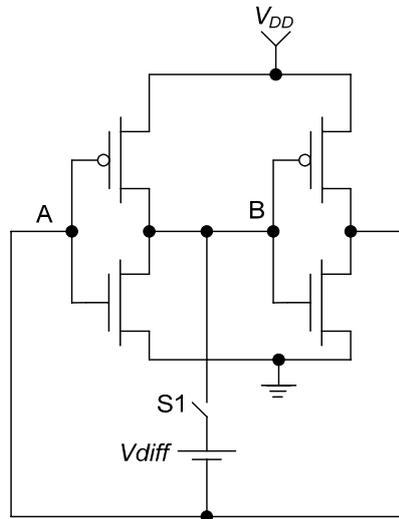
**Figure 2 Typical metastability simulation circuit**
