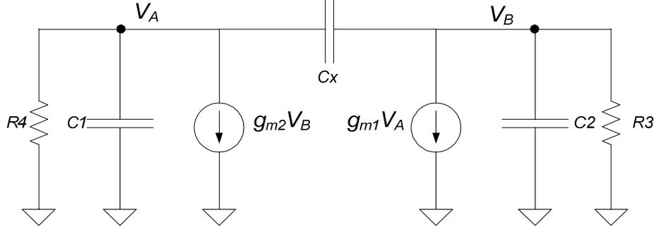
**Figure 11 Basic model of the symmetric boost latch with gate-drain capacitance**
