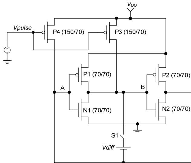
**Figure 13 Symmetric boost latch - simulation circuit**
