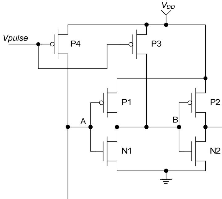
Figure 9 Symmetric boost latch
