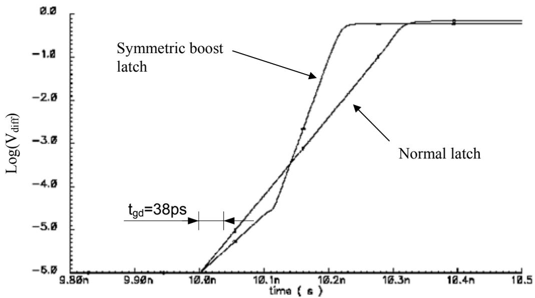
Figure 21  $\tau$  calculation,  $V_{DD}=0.7V$ ,  $T=-20^{\circ}C$ .  $\tau$  (symmetric boost)=11ps,  $\tau$  (Normal latch)=24ps.
