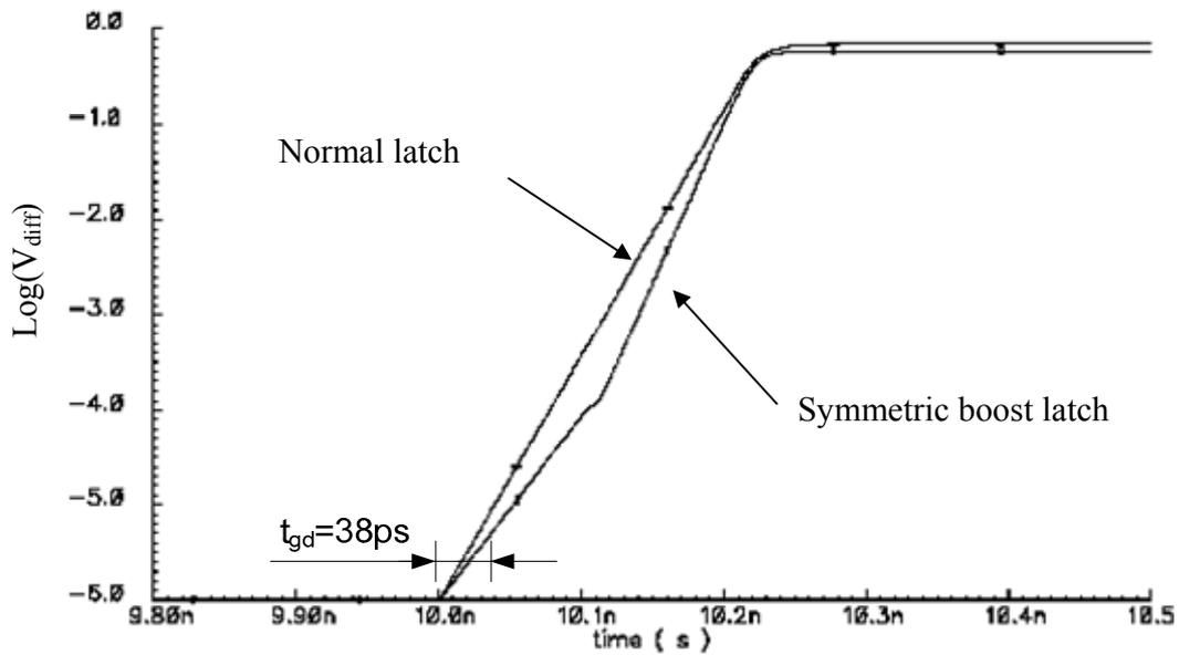
Figure 15  $\tau$  calculation,  $V_{DD}=0.7\text{V}$ ,  $T=27^\circ\text{C}$ .  $\tau$  (symmetric boost)=13ps,  $\tau$  (Normal latch)=16ps.
