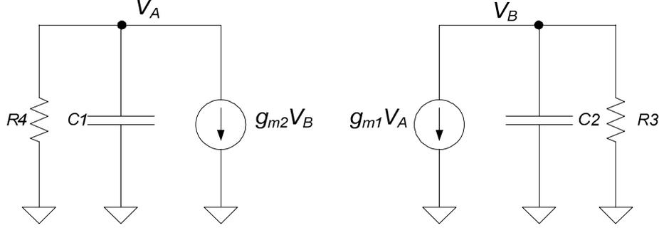
**Figure 10 Basic model of the Symmetric boost latch**
