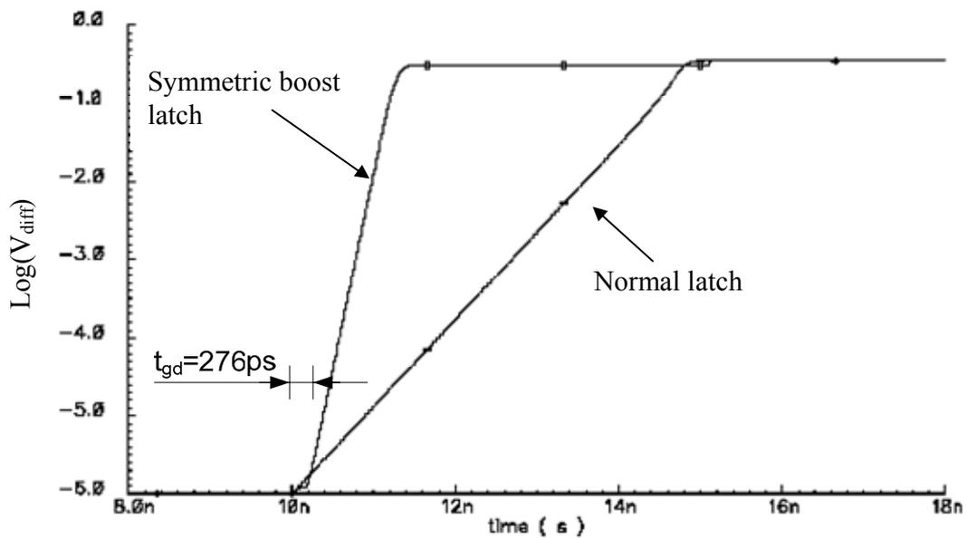
Figure 19  $\tau$  calculation,  $V_{DD}=0.35V$ ,  $T=27^{\circ}C$ .  $\tau$  (symmetric boost)=87ps,  $\tau$  (Normal latch)=388ps.
