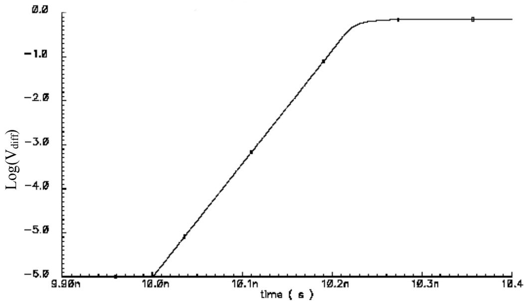
Figure 4 Logarithmic voltage difference.  $\tau$  is the inverse of the slope of the straight segment
