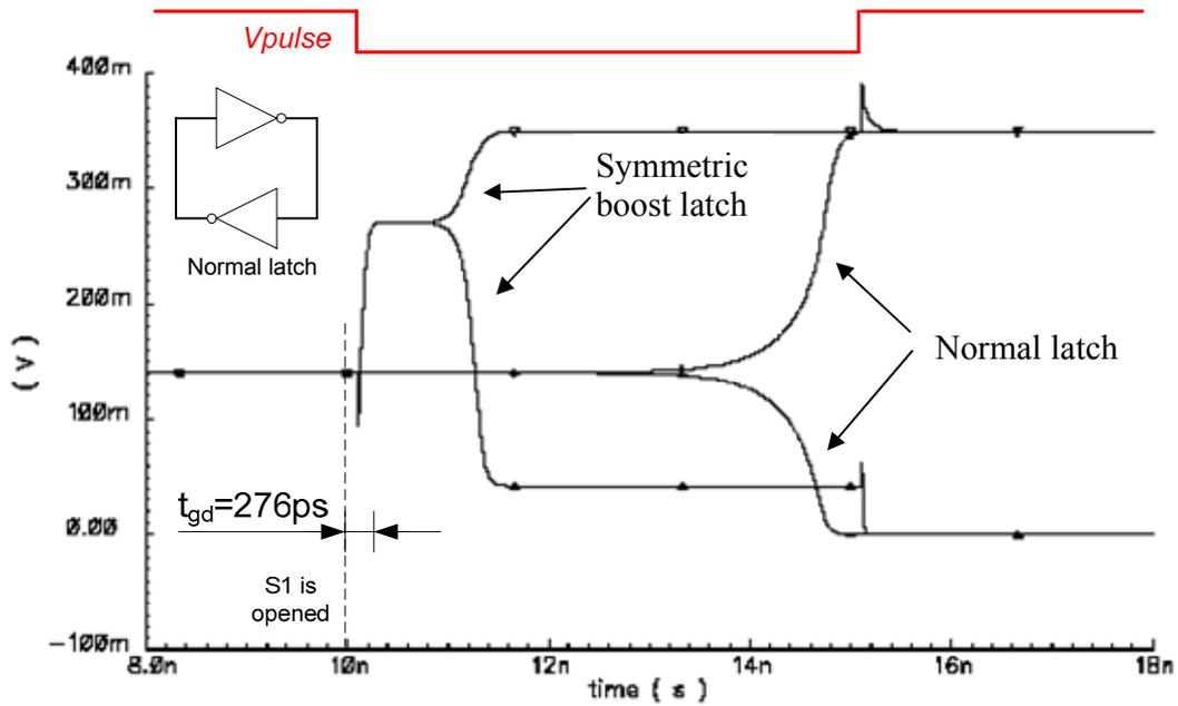
Figure 18 Transient analysis,  $V_{DD}=0.35V$ ,  $T=27^{\circ}C$
