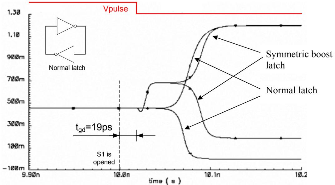
Figure 27 Transient analysis,  $V_{DD}=1.2V$ ,  $T=27^{\circ}C$
