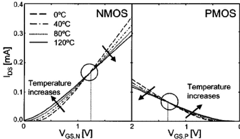
Figure 5 Measured temperature dependence for NMOS and PMOS transistors, temperature range from 0 to 120° C (adapted from [13])
