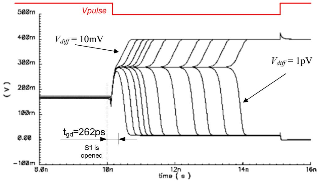
Figure 26 Transient analysis of the symmetric boost latch,  $V_{DD}=0.4V$ ,  $T=-20^{\circ}C$
