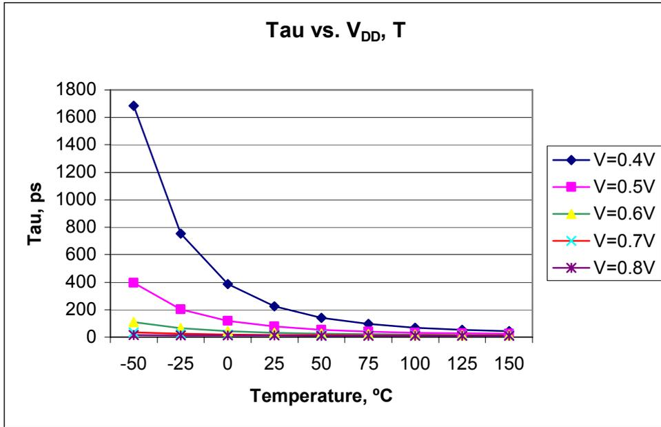
Figure 7  $\tau$  dependence on  $V_{DD}$ , T
