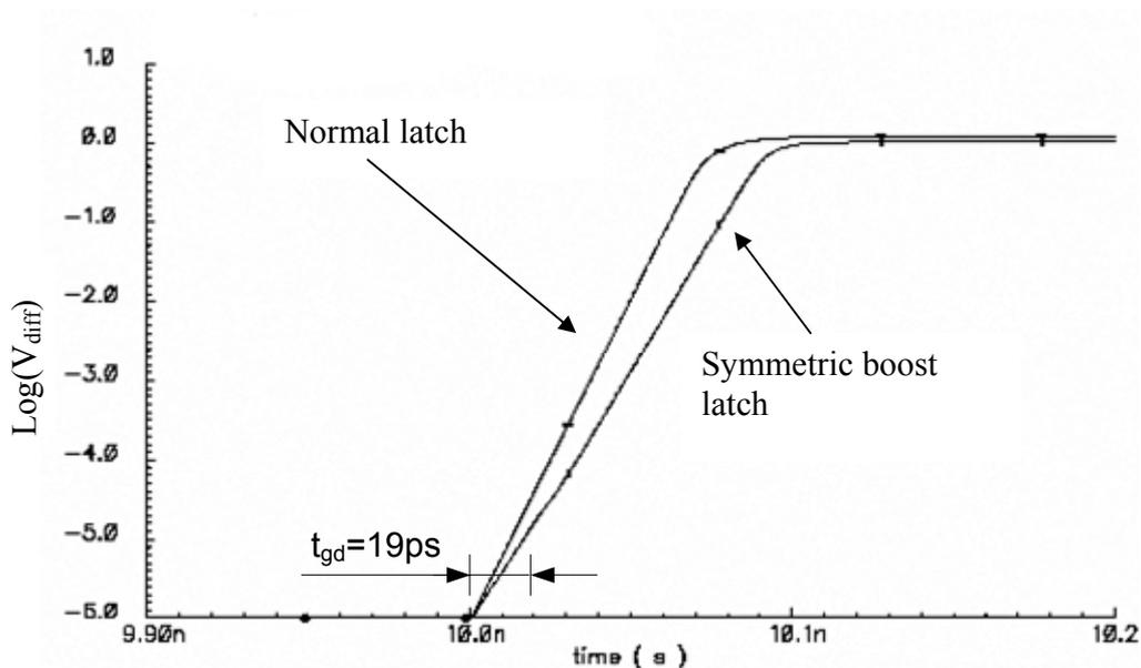
Figure 28  $\tau$  calculation,  $V_{DD}=1.2V$ ,  $T=27^{\circ}C$ .  $\tau$  (symmetric boost)=6.4ps,  $\tau$  (Normal latch)=5.1ps.
