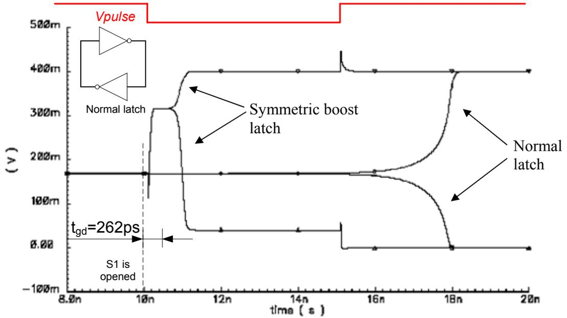
Figure 22 Transient analysis,  $V_{DD}=0.4V$ ,  $T=-20^{\circ}C$
