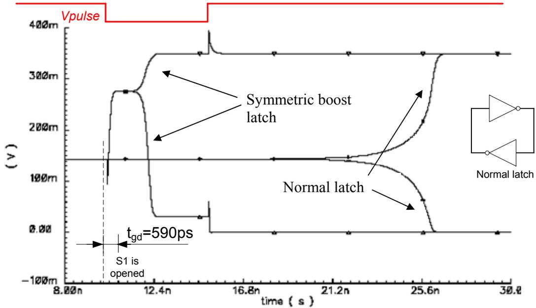
Figure 24 Transient analysis,  $V_{DD}=0.35V$ ,  $T=-20^{\circ}C$
