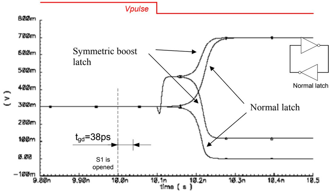
Figure 14 Transient analysis,  $V_{DD}=0.7\text{V}$ ,  $T=27^\circ\text{C}$
