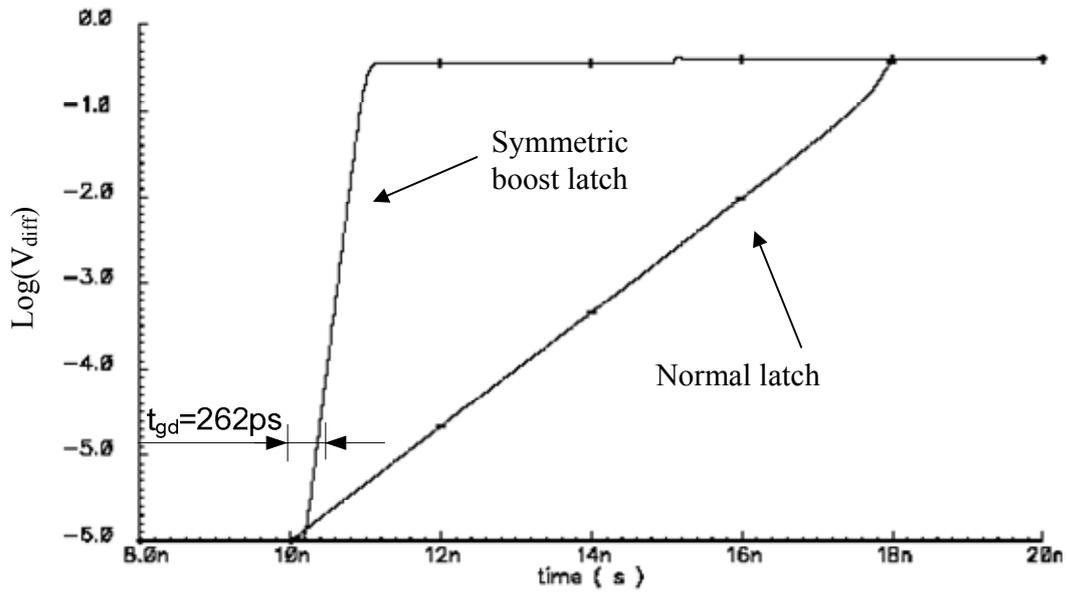
Figure 23  $\tau$  calculation,  $V_{DD}=0.4V$ ,  $T=-20^{\circ}C$ .  $\tau$  (symmetric boost)=63ps,  $\tau$  (Normal latch)=651ps.
