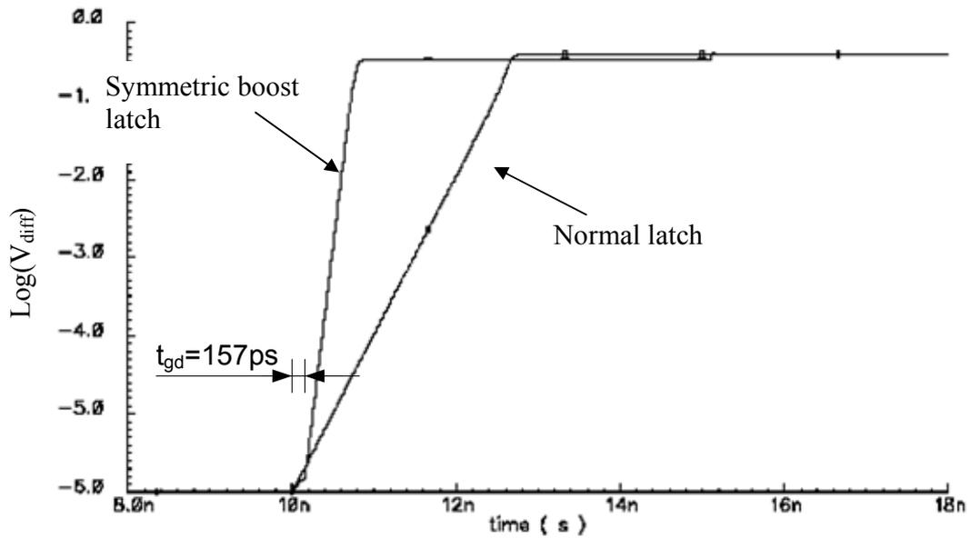
Figure 17  $\tau$  calculation,  $V_{DD}=0.4V$ ,  $T=27^{\circ}C$ .  $\tau$  (symmetric boost)=50ps,  $\tau$  (Normal latch)=214ps.
