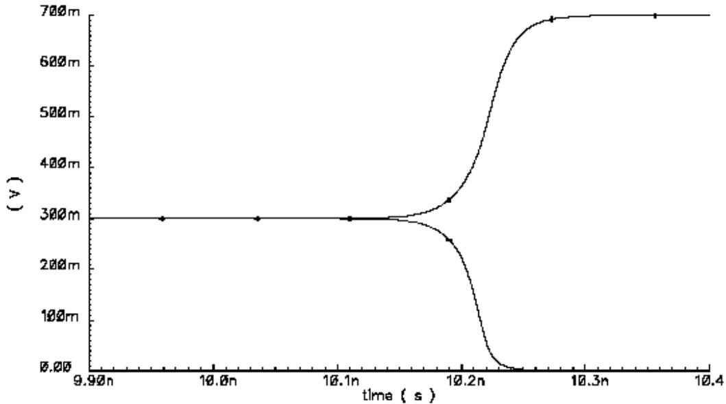
Figure 3 Voltage waveform of the diverging nodes of the latch
