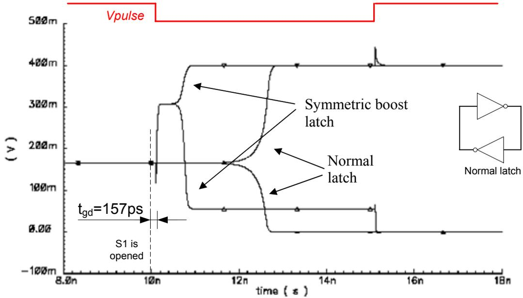
Figure 16 Transient analysis,  $V_{DD}=0.4V$ ,  $T=27^{\circ}C$
