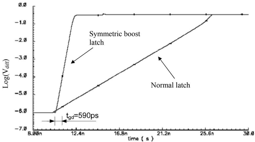
Figure 25  $\tau$  calculation,  $V_{DD}=0.35V$ ,  $T=-20^{\circ}C$ .  $\tau(\text{symmetric boost})=144ps$ ,  $\tau(\text{Normal latch})=1332ps$ .
