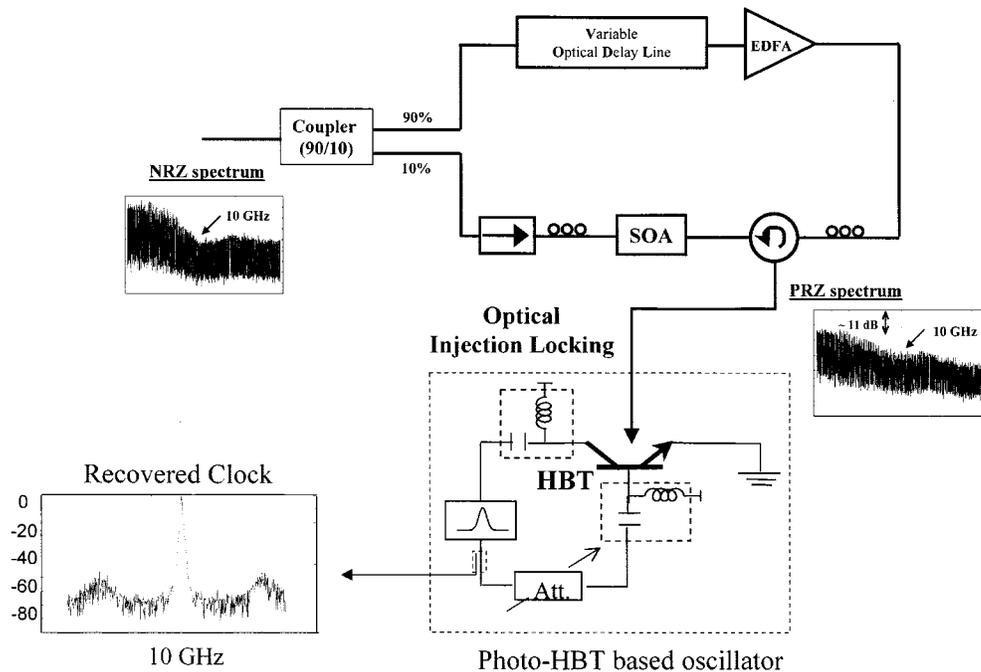
Fig. 1. Experimental schematic of the all-optical processing system and the photo-HBT-based oscillator.
