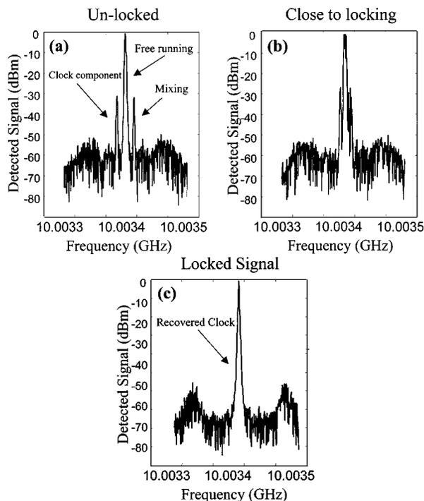
Fig. 4. Optical injection locking sequence. (a) Unlocked case. (b) Close to locking. (c) Locked case.
