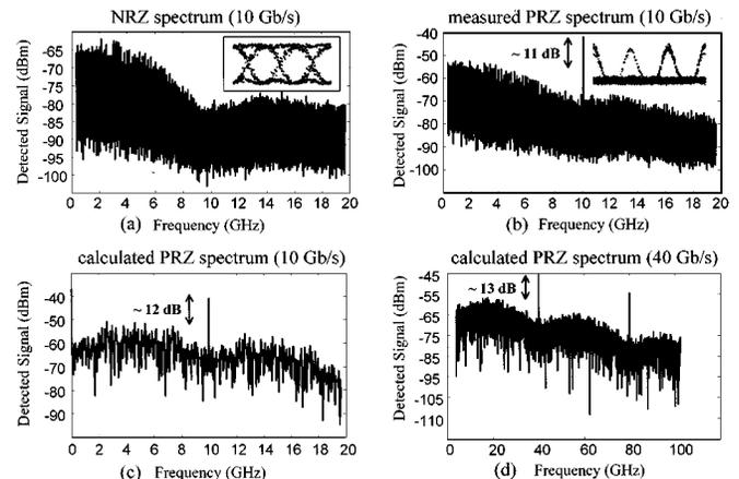
Fig. 3. Detected spectra: (a) Spectrum of the incoming 10-Gb/s NRZ signal. (b) Measured spectrum of the all optically processed signal. (c) Simulated spectrum of the all optically processed 10-Gb/s signal. (d) Simulated spectrum of the all optically processed 40-Gb/s signal.
