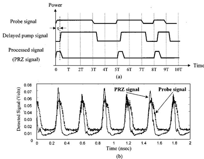
Fig. 2. (a) Time domain all optical processing principle of operation. (b) Measured example with a 10-Gb/s "100" sequence.
