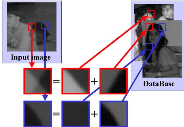
Figure 4: Optimization by discretization into patches. For each input patch we search a database of photographs for pairs of similar patches and use these to define a discrete optimization problem.
