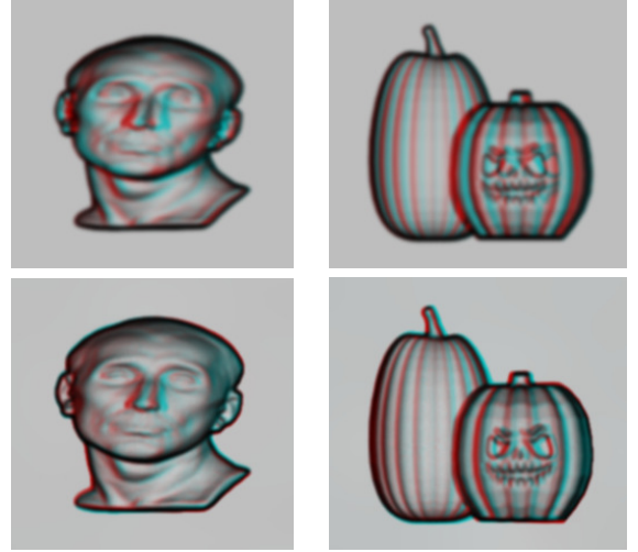
Figure 9: The leftmost and rightmost viewpoints of synthetic surfaces superimposed in different color channels. Our display (2nd row) produces weaker disparity compared to the target (top row) due to neighborhood averaging of the 1st layer power.
