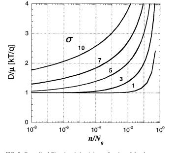
FIG. 5. Generalized Einstein relation ( $\eta$ ) as a function of the charge concentration for a variety of disorder parameters (calculated based on Ref. 23);  $N_0$  is the total DOS.
