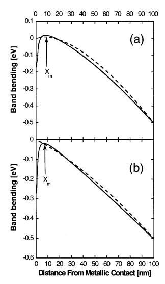
FIG. 2. Typical band bending. The barrier heights are (a) 0.2 and (b) 0.3 eV, respectively. The voltage applied is 0.5 V beyond the flat band condition (i.e.,  $V \sim 2.5$  V). The dashed line was calculated using the "standard" (lumped) model and the solid line using our explicit model.
