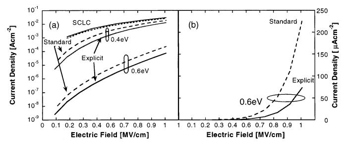
FIG. 4. (a) Current density as a function of the mean field for a 100 nm long device and varying injection barriers of 0.2, 0.4, and 0.6 eV and device length of 0.1  $\mu$ m. (b) Current density for a 0.6 eV barrier on a linear scale. Standard = Lumped model; explicit = our model; SCLC = space charge limited current as in Eq. (3).
