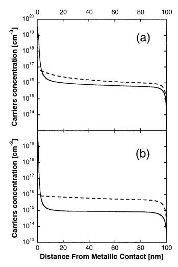
FIG. 3. Charge density distribution for contact injection barriers of (a) 0.2 and (b) 0.3 eV. The dashed line was calculated using the "standard" (lumped) model and the solid line using our explicit model.
