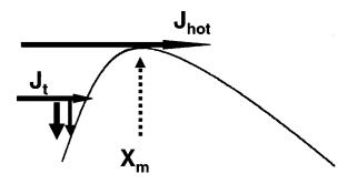
FIG. 1. Schematic of the contact region.  $x_m$  is the coordinate of peak of the image force potential in the presence of an applied field,  $J_t$  is the current of carriers thermalized at the contact region,  $J_h$  is the current of "hot" carriers that successfully overcome the peak ballistically.
