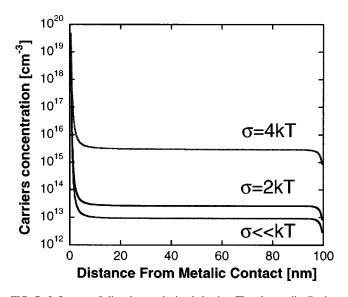
FIG. 7. Influence of disorder on device behavior. The charge distribution and I-V curve show a significant variety for difference disorder in hopping site energies.
