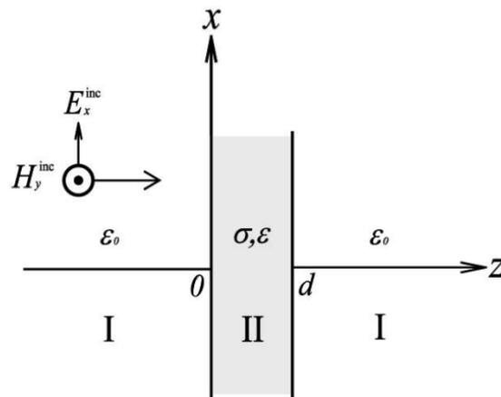
Fig. 1. Interaction of EM plane wave with a conducting layer (region II).
