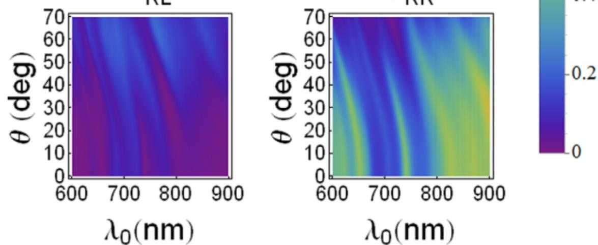
**Figure 6** Measured spectrums of the four circular transmittances of the dual-band circular-polarization filter for  $\theta \in [0^\circ, 70^\circ]$ . [Color figure can be viewed in the online issue, which is available at [wileyonlinelibrary.com](http://wileyonlinelibrary.com).]
