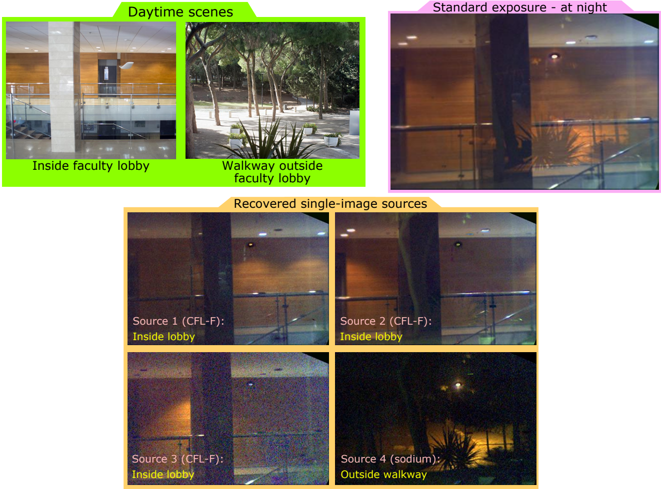
Fig. 4. Semi-reflection separation for an AC-illuminated scene experiment. An indoor scene is illuminated by CFL-F bulbs, each connected to an arbitrary AC phase \phi \in \mathbb{P} . The ACam is placed inside the lobby, facing outside. The indoor scene in (a) is semi-reflected by a lobby glass door. The outdoor scene the camera is facing is (b). At night, the outdoor scene is illuminated by a Sodium lamp. A standard exposure image shows a mixture of the semi-reflected and transmitted components. ACam captured a K = 26 sequence using C = 1200 and a camera gain of 25 (see video in [10, 11]). The scene was unmixed using S = 4 source taken from DELIGHT.
