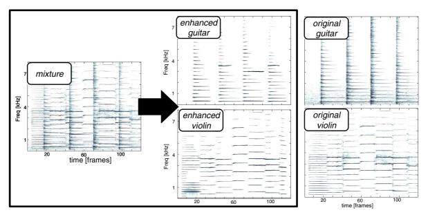
Figure 2. Spectrograms corresponding to the violin-guitar sequence. Darker points in each plot indicate a higher energy content, as a function of t and f. Based on *visual* data, the audio components of the violin and guitar were automatically separated from a soundtrack, which had been recorded by a *single* microphone. [Right] The true components of each instrument, acquired separately. You may listen to the results via the link *www.ee.technion.ac.il/~yoav/research/harmony-in-motion.html*
