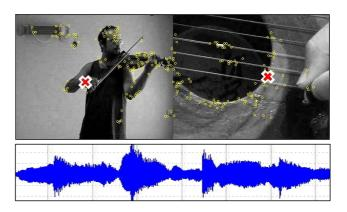
Figure 1. A frame and the audio from the violin-guitar movie. A camcorder and a single microphone were used. Two movies were compounded and then processed as a whole. Out of the selected and tracked visual features [Dots], two are automatically associated to the audio [Crosses]: correctly, one per source. The audio mixture is also decoupled to a guitar and a violin. See/hear this via *www.ee.technion.ac.il/~yoav/research/harmony-in-motion.html*
