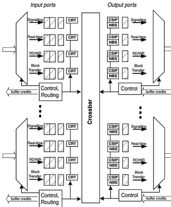
Fig. 5. Router architecture.
