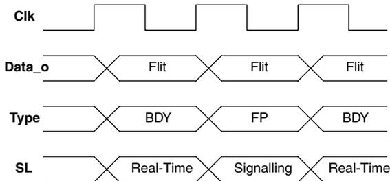
Fig. 6. Tx waveforms: a *Real-Time* packet is pre-empted by a single-flit *Signaling* packet.
