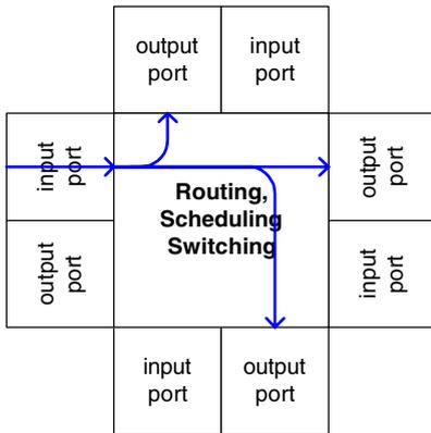
Fig. 4. Router—data flow.
