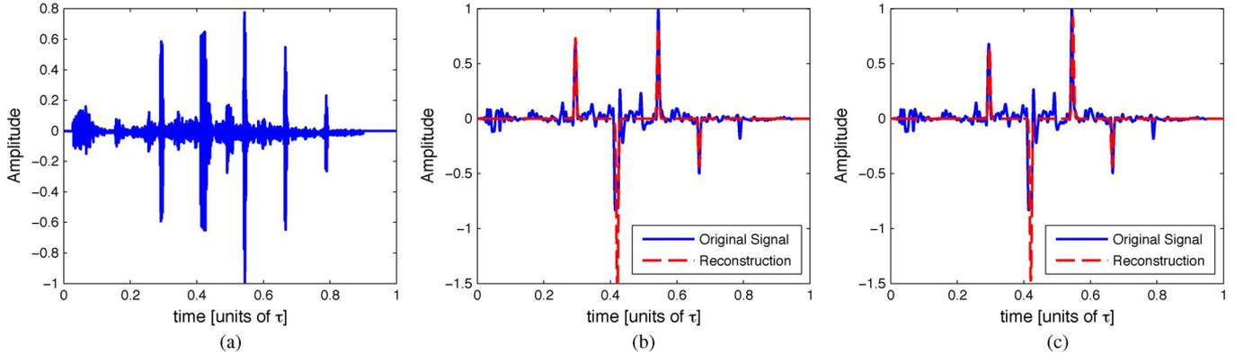
Fig. 17. Applying the SoS sampling scheme with  $b_k = 1$  on real ultrasound imaging data. Results are shown versus original signal which uses 4160 samples. (a) Recorded ultrasound imaging signal. The data was acquired by GE healthcare's Vivid-i ultrasound imaging system. Reconstructed signal (b) using  $N = 17$  samples and (c) using  $N = 33$  samples (taken from [163]).
