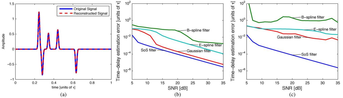
Fig. 15. Performance comparison of finite pulse stream recovery using Gaussian [6], B-spline, E-spline [7], and SoS sampling kernels. (a) Reconstructed signal using SoS filters versus original one. The reconstruction is exact to numerical precision. (b)  $L = 3$  Dirac pulses are present, (c)  $L = 5$  pulses (taken from [163]).
