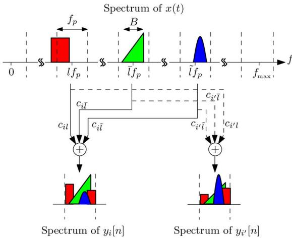
Fig. 12. Spectrum slices of  $x(t)$  are overlaid in the spectrum of the output sequences  $y_i[n]$ . In the example, channels  $i$  and  $i'$  realize different linear combinations of the spectrum slices centered around  $lf_p$ ,  $lf_p$ ,  $lf_p$ . For simplicity, the aliasing of the negative frequencies is not drawn (taken from [9]).
