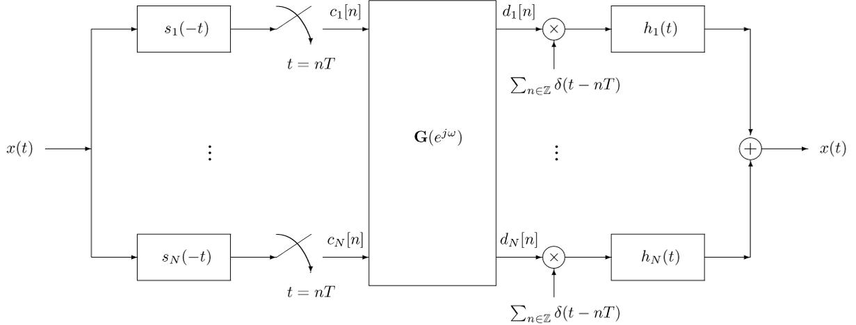
Fig. 11. Sampling and reconstruction in shift-invariant spaces. A compressive signal acquisition scheme can be obtained by reducing the number of sampling filters from  $N$  to  $p < N$  and replacing the filter bank  $\mathbf{G}(e^{j\omega})$  with a CTF block with real-time recovery (taken from [18]).
