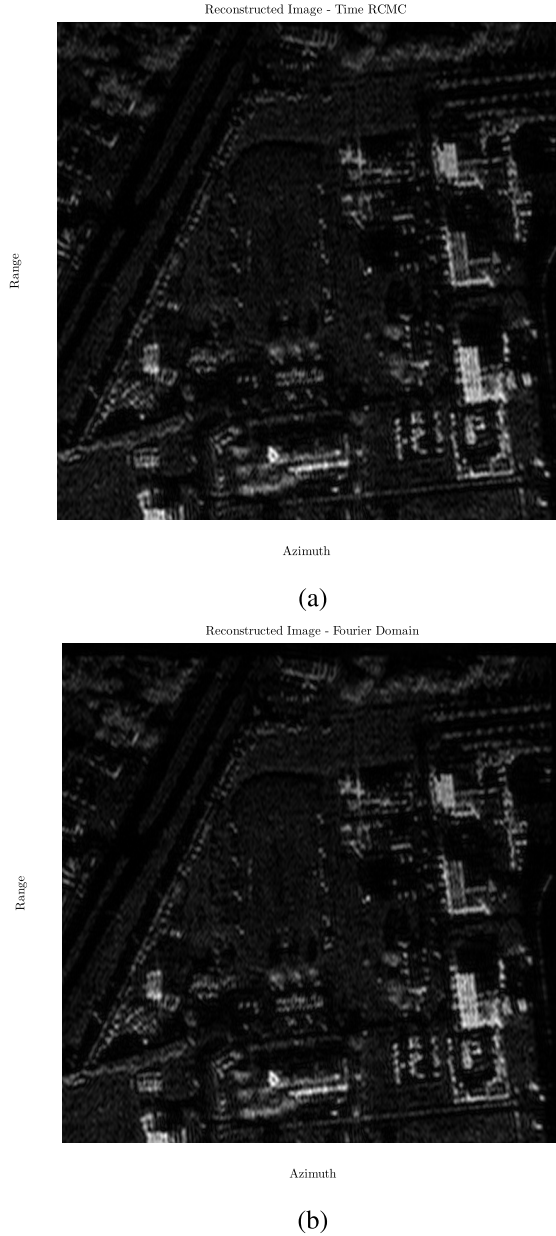
Fig. 7. Comparison between two reconstructed images. (a) Conventional RDA using oversampled raw data. (b) Fourier RDA, |v(k, l)| = 5 , with no oversampling.
