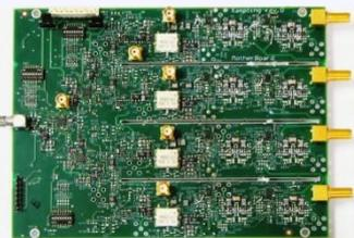
$m = 4$  channels, sampling rate = 70 MHz/channel
