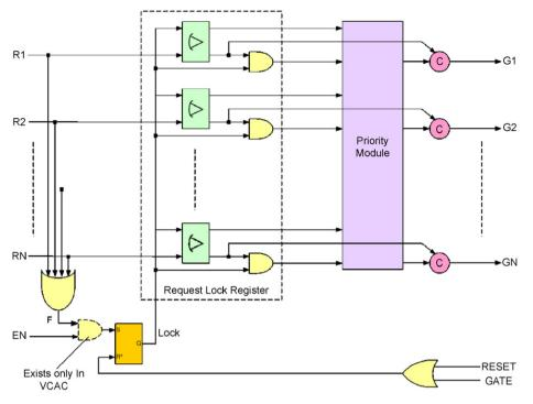
Fig. 12. *N*-way static priority arbiter.
