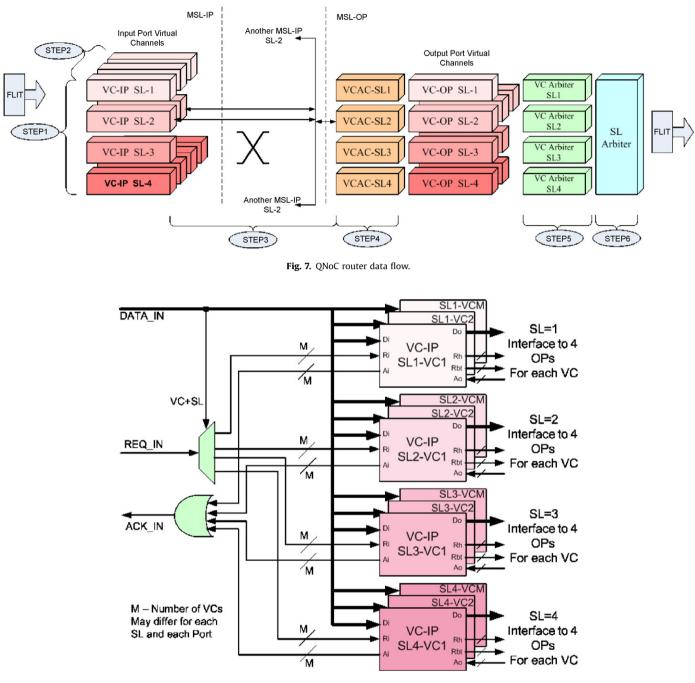
Fig. 8. QNoC multi-service levels router input port.
