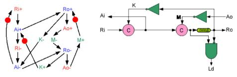
Fig. 10. Latch-control circuit and STG.
