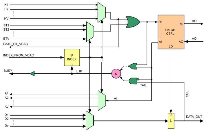
Fig. 17. Virtual channel output port (VC-OP) architecture.
