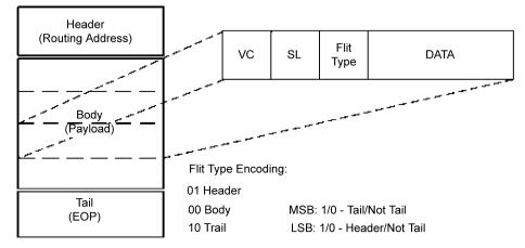
Fig. 6. Packet structure and flit format.
