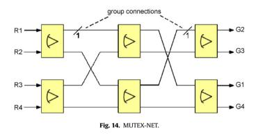
The header request arbitration is performed by a MUTEX-NET, which is faster than the tree-arbiter while still incurring similar latency and area [10].
