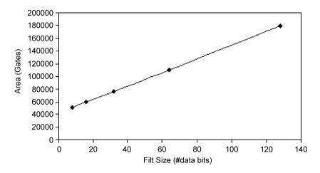
Fig. 20. Router cell area dependence on flit size.
