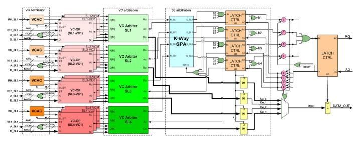
Fig. 11. QNoC multi-service level router output port (M-way VC arbiters are used in VC arbitration stage, K-way SPA is used in SL arbitration stage). In this figure K = 4, M = 3.
