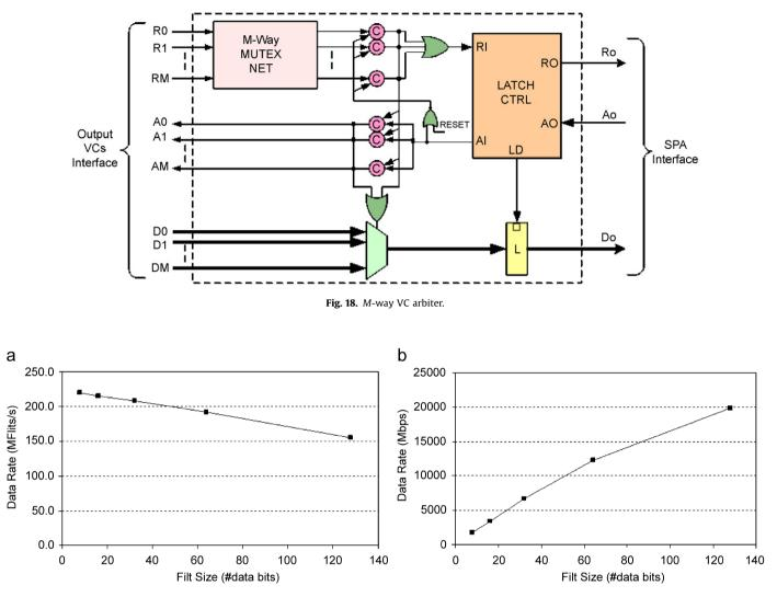
Fig. 19. Router throughput dependence on flit size: (a) flit rate, (b) bit rate.
