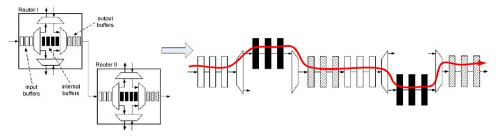
Fig. 3. NoC data path as pipeline.
