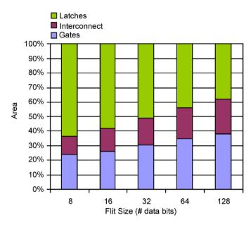
Fig. 21. Area distribution. Switching gates and wires dominate the area as flit size grows.
