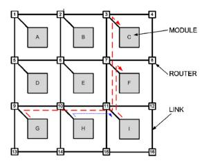
Fig. 1. QNoC 2D mesh architecture and the impact of service level preemption.
