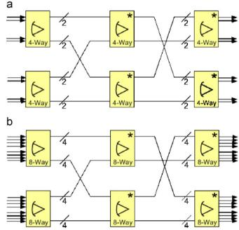
Fig. 15. N-way MUTEX-NET. (a) 8-way MUTEX-NET example (b) 16-way MUTEX-NET example.
