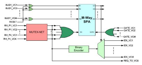
Fig. 13. Virtual channel admission control (VCAC) module.
