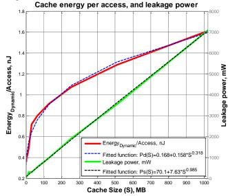
Figure 3. Cache dynamic read energy/access vs. cache size (CACTI-6).
