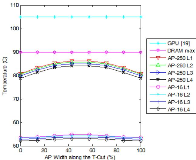
Fig. 6. Temperatures in four silicon layers along the T-Cut (cf. Fig. 3(a)) for 16 mm<sup>2</sup> and 250 mm<sup>2</sup> APs
