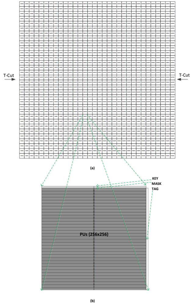
Fig. 3. AP floorplan for HotSpot thermal modeling
