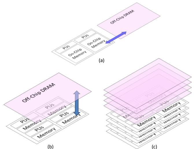
Fig. 1. Architecture evolution: (a) 2D PU array with on-chip and off-chip memory, (b) stacked PU array and DRAM dies, (c) 3-D multilayer PU/AP with multilayer DRAM
