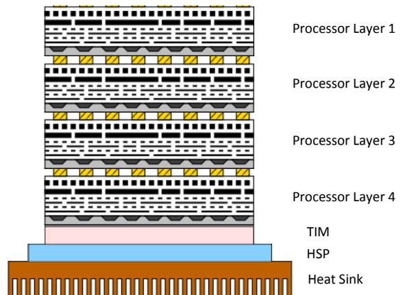
Fig. 4. 3-D thermal model (based on [11])
