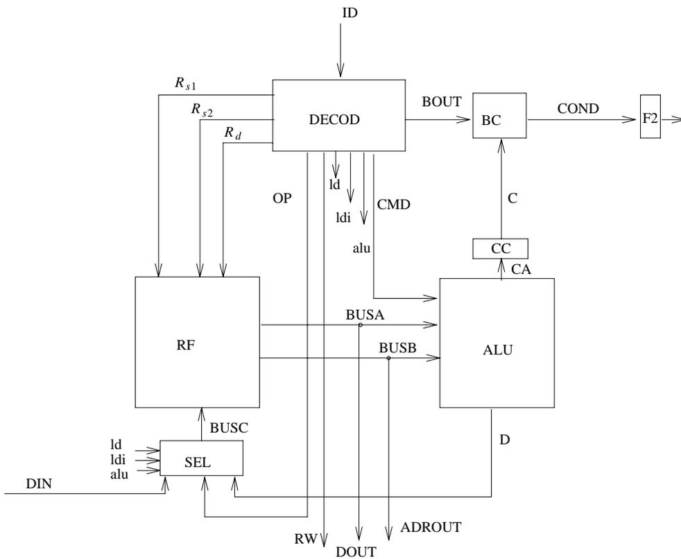
Figure 6. The data processor
