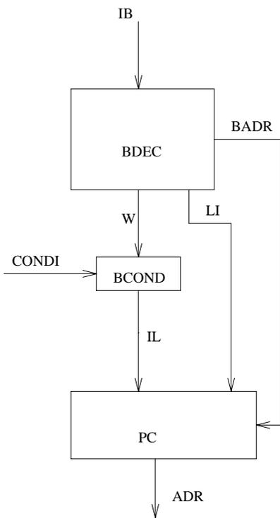
Figure 8. The branch processor
