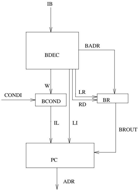
Figure 12. The delayed-branch branch processor (substituting Figure 8)
