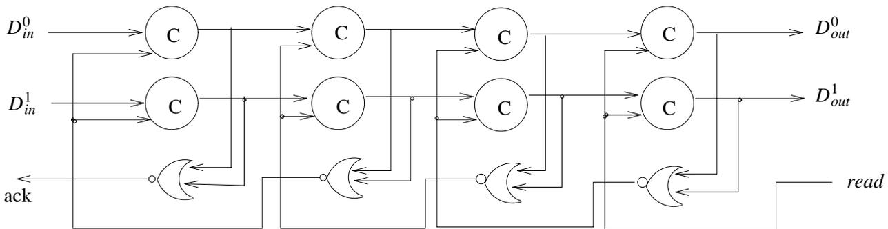
Figure 10: A four-stage self-timed FIFO
