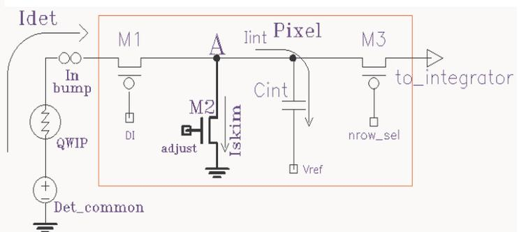
Fig. 4: Current readout architecture: The front-end is similar to the voltage readout scheme; the output current flows through a row-select transistor. The reset of  $C_{int}$  is part of the readout operation.
