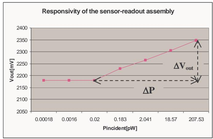
Fig. 10: Output voltage of the QWIP-readout cell assembly as a function of radiation power incident upon a QWIP at  $84^0K$ , with  $200 \times 200 \mu m^2$  active area, positioned at 7cm from a black-body of  $1000^0K$
