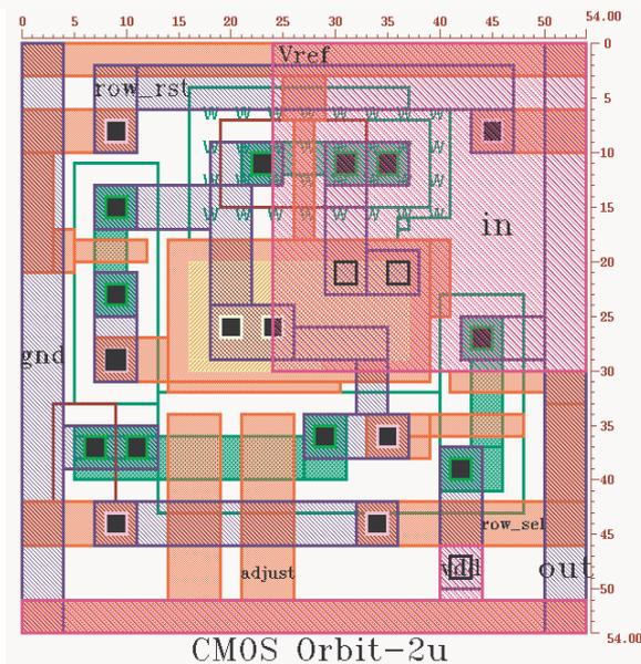
Fig. 5: Layout of a self-cascode skimming, voltage-readout pixel
