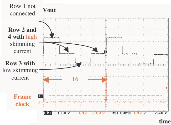
Fig. 7: Current readout array's serial output, with four identical pixels in a row and seeing the same background ( $I_{dc}=10\mu A$ )
