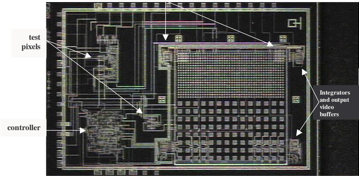
Fig. 11: Micro-Photograph of the prototype integrated circuit
