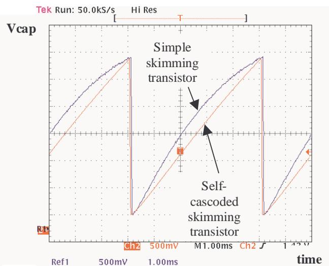
Fig. 8: Improved linearity of integration in the case of self-cascoded skimming transistor is demonstrated by measuring the voltage on the capacitor between two consecutive resets
