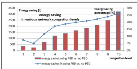
Figure 6. Energy savings at various congestion levels for PBD and no PBD
