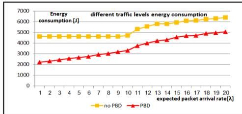
Figure 3. Various traffic levels energy consumption
